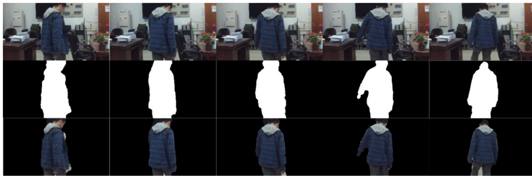
Figure 9. The target area extraction results of 80~84 frames. From top to bottom are the corrected images, the moving target binarized image extracted by the target detection method in this paper, the superimposed display of the binarized image, and the corrected image.
