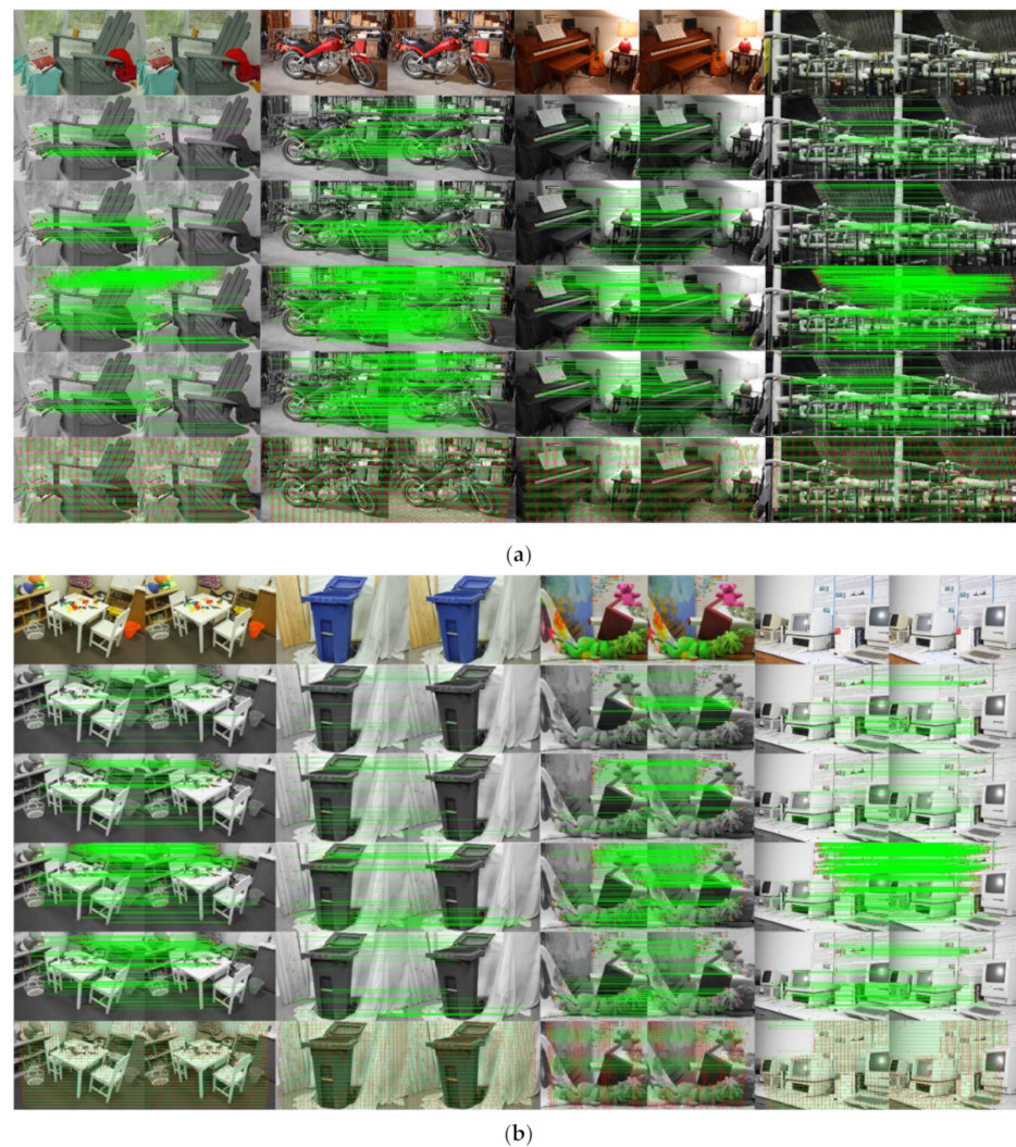
Figure 7. Middlebury Stereo Datasets stereo matching results. (a) From left to right are the Adirondack, Motorcycle, Piano and Pipes stereo image pairs; (b) from left to right are the PlayTable, Recycle, Teddy and Vintage stereo image pairs; (a,b) from top to bottom are the stereo image pair, stereo-Fast, stereo-Harris, stereo-Sift, stereo-Surf, and stereo deep matching results.
