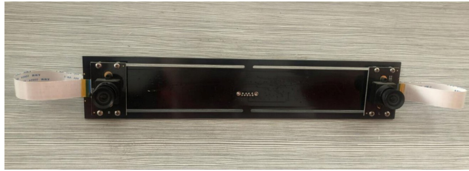
Figure 8. Parallel structure of the binocular camera.
