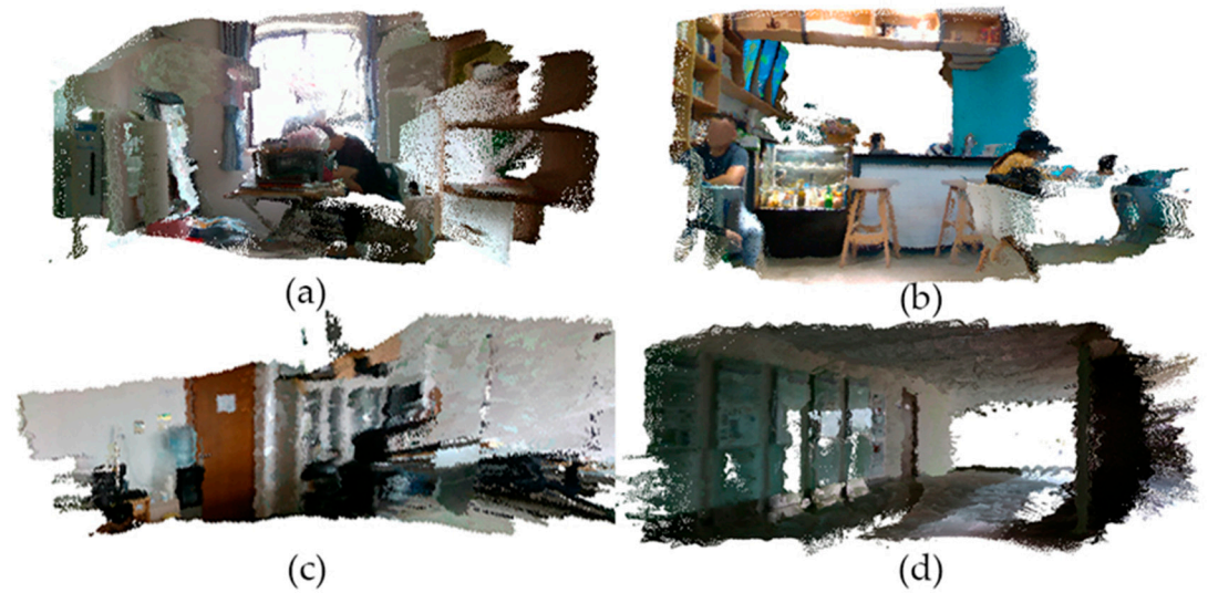
Figure 3. Three-dimensional model constructed from RGB-D image: (a) Home scene; (b) cafe scene; (c) office scene; (d) corridor scene.
