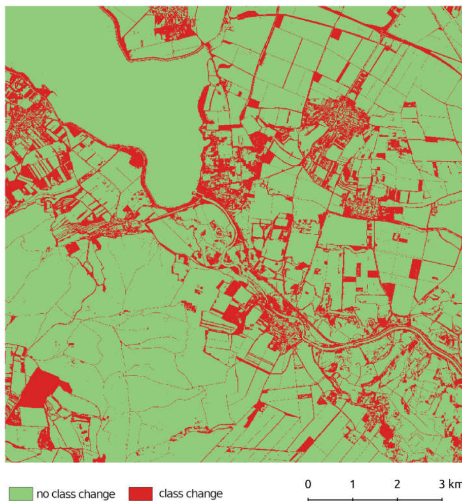
Figure 7. Monitoring class mismatch between the original cadastral data and the LightGBM prediction to visually assess the results of the classification. Sources: Sentinel-2 imagery from 30.3 to 16.10.2019 [80], Czech cadastral map [85].
