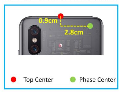
Figure 8. The position of the Xiaomi MI8's phase center.
