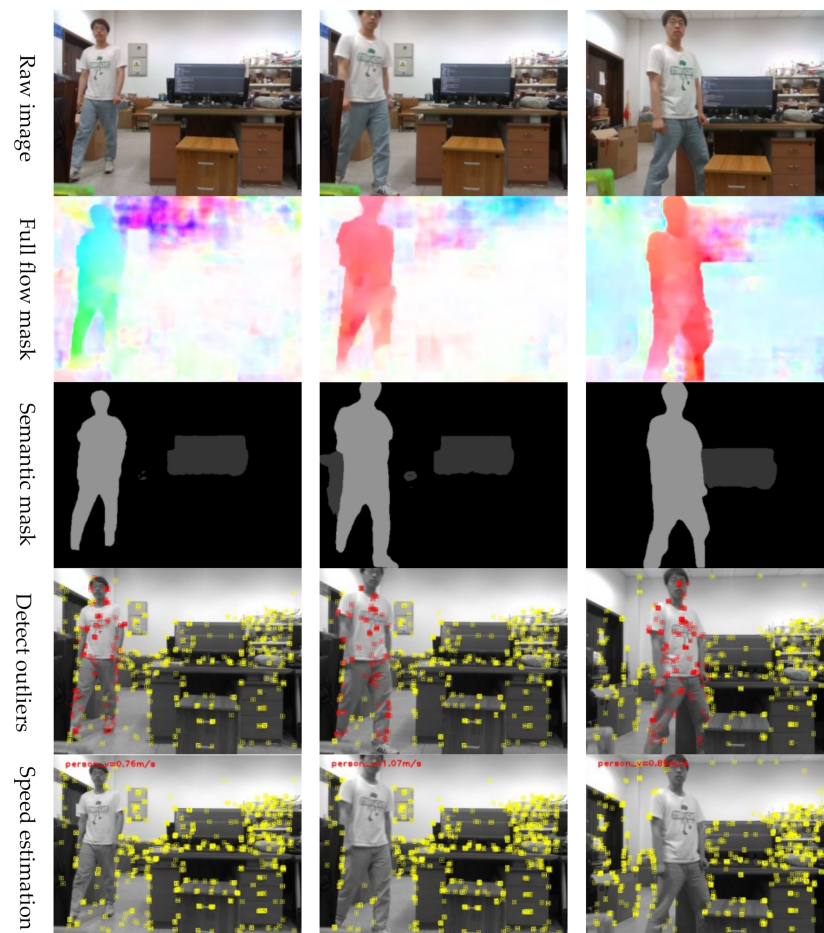
Figure 9. Real environment experiments conducted with a live RGB-D camera under physical conditions. The first row presents the raw RGB images and the second row shows the full optical flow as predicted by PWC-Net. The third row is the semantic mask, and the fourth row indicates that our system can separate the dynamic keypoints from real-world conditions. The final row demonstrates the determination of the speed of dynamic objects after the removal of outliers.
