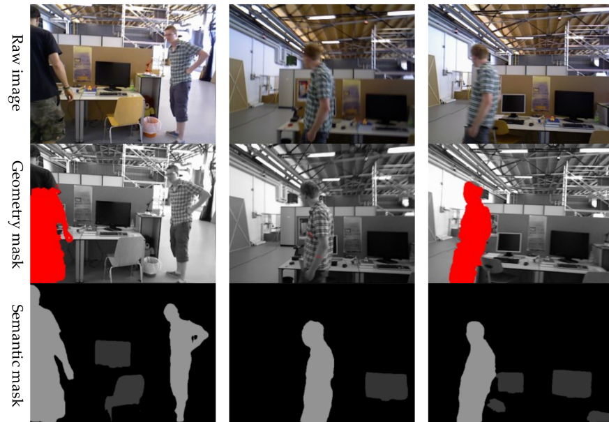
Figure 6. Examples of the results of geometric and semantic segmentation modules on a Technische Universität München (TUM) fr3/walking/xyz sequence. The first row presents the raw RGB images. The second and third rows present the results of the geometric and semantic segmentation modules, respectively. Of note, the second column indicates how the epipolar constraint can further identify dynamic points when the optical flow residuals become invalid.
