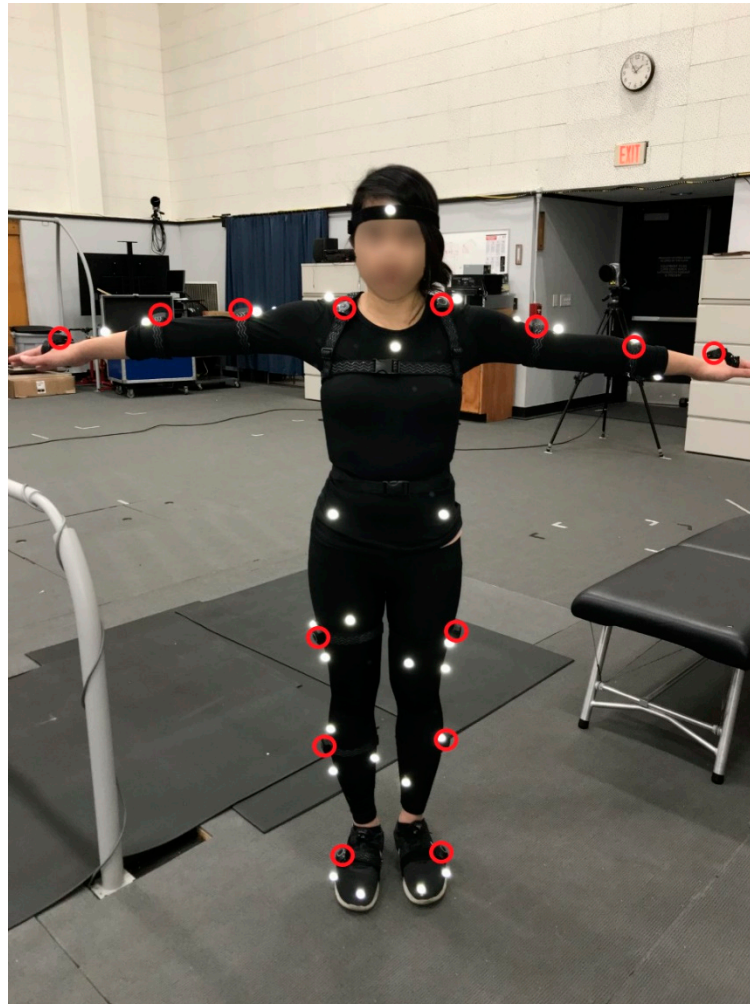
Figure 5. Subject preparation. Locations of the experimental motion capture reflective markers and Perception Neuron Pro IMU suit. IMUs are circled in red.
