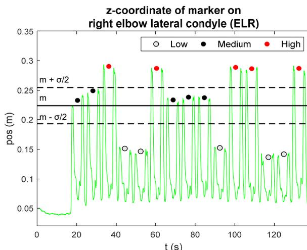
**Figure 5.** Algorithm for the distinction among pick and place gestures. Three horizontal black lines are inserted: a continuous line ( $m$ ) and two dashed lines ( $m \pm \sigma/2$ ). The mean values of each pair of peaks are represented through dots recalling the boxes’ colors.
