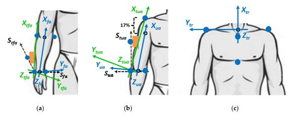
**Figure 4.** Anatomical reference systems (blue) and technical reference systems (green) defined from markers coordinates: (a) right forearm systems; (b) right upper arm systems; (c) trunk system.
