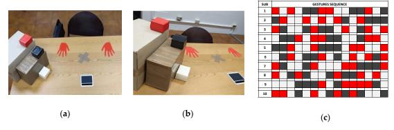
**Figure 2.** Top view (**a**) and perspective view (**b**) of the setup adopted for the test. Three colored boxes at different heights (white = low, black = medium, red = high); hand silhouettes indicating hands neutral position and the cross marking the box placement on the table are visible; (**c**) table of the randomized sequence of pick and place gestures.
