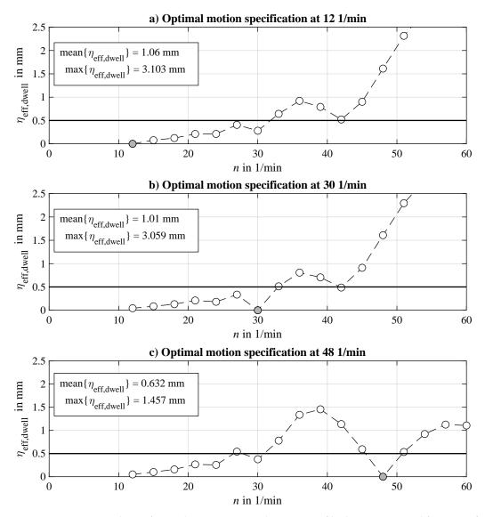
**Figure 5.** Process simulation for applying one optimal motion profile that is optimized for a specific operating speed and scaled to other operating speeds. Three results, which differ in the operating speed for which the motion profile is optimized, are displayed: 121/min (**a**), 301/min (**b**), and 481/min (**c**).
