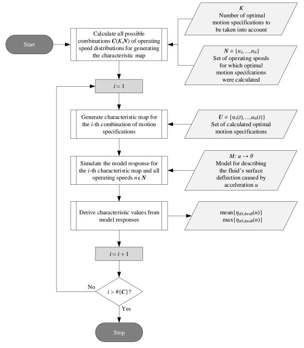
**Figure 8.** Algorithm for evaluating all possible distributions of optimal motion specifications to generate a characteristic map for a given set *N* of operating speeds and number *K* of motion specifications to be considered. For each generated map, the characteristic values are evaluated from a simulation run.
