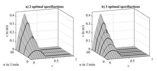
**Figure 6.** Discrete execution of operating-speed-dependent motion profiles for two (**a**) and three (**b**) optimal specifications whereby each motion profile is scaled proportional to the operating speed. Exemplarily, the characteristic map of the velocity is displayed with obvious discontinuities.
