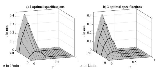
**Figure 7.** Continuous execution of operating-speed-dependent motion profiles for two (**a**) and three (**b**) optimal specifications by linear interpolation in the direction of the operating speed. Obviously, no discontinuities occur in the characteristic map.
