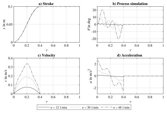
**Figure 4.** Stroke (**a**), velocity (**c**), and acceleration (**d**) graphs of the optimized motion specifications resulting from solving the corresponding optimal control problems for three different operating speeds. The simulated model responses are also displayed (**b**). Obviously, no residual vibration is achieved, which must be why the optimization was successful. For a better comparison, the motion profiles are displayed over their normalized time  $\tau = t/T_{cycle}$ .
