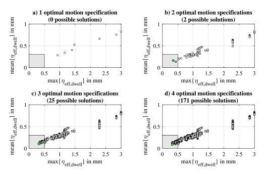
**Figure 11.** Determining the best distribution of optimal motion profiles for different numbers of specifications. A solution is feasible, if the characteristic values are inside the gray rectangular box. From all solutions, the best solution, which exhibits the smallest distance to the origin, is chosen. One (**a**), two (**b**), three (**c**), and four (**d**) optimal motion profiles are considered.
