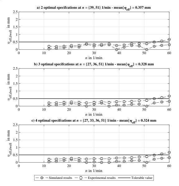
**Figure 13.** Comparison of simulated and experimental results for applying linear interpolated and optimal operating-speed-dependent motion profiles for controlling liquid slosh. The measure for the residual vibration  $\eta_{\text{eff,dwell}}$  is displayed for different numbers of optimal motion specifications: two (**a**), three (**b**), and four (**c**) optimal motion profiles are considered for generating the characteristic map.
