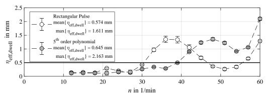
**Figure 10.** Experimental results by applying the rectangular pulse motion profile and a 5th order polynomial motion profile for operating speeds *n* ranging from 12 to 60 1/min. The characteristic value  $\eta_{\text{eff.dwell}}$  is a measure for the residual vibration of the fluid surface.
