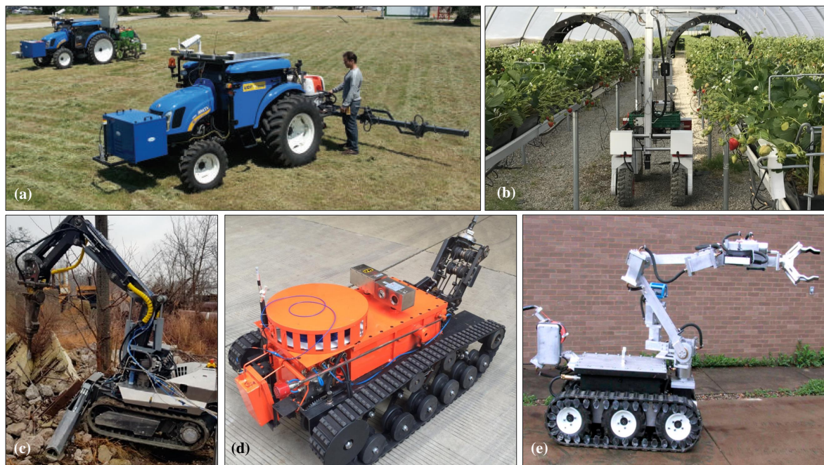
Figure 1. Example field robotic platforms for (a)–(b) agriculture [28,29], (c) construction and demolition [40], (d) search-and-rescue [43], and (e) working in explosive or hazardous environments [46] (All figures originally published under CC-BY-4.0 license).
