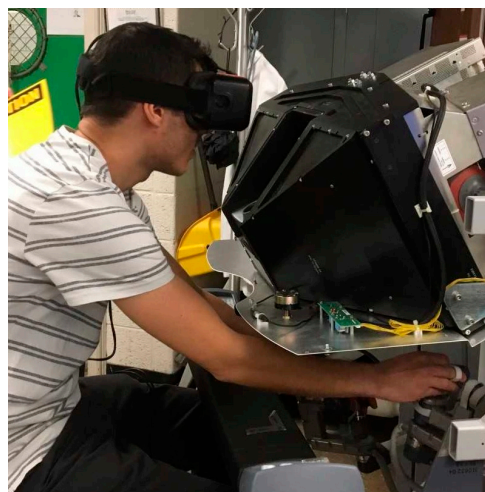
Figure 8. A user controlling da Vinci ECM using HMD. The cover of the surgeon console is removed to allow more room for the head movements.
