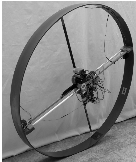
Figure 1. The OSU Roller has a mass of 0.950 kg with a perimeter of 2.095 m.
