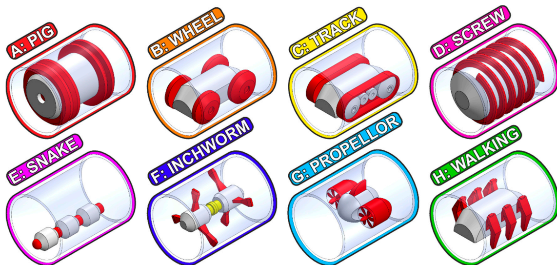
Figure 3. The eight main elements of in-pipe robotic locomotion (A–H).
