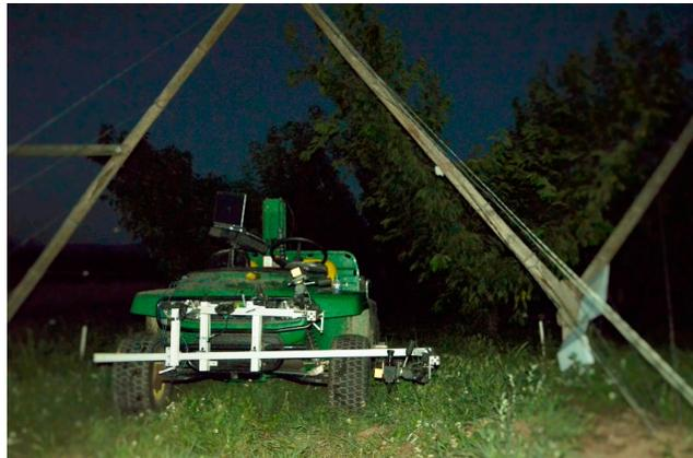
**Figure 2.** Setup for imaging cherry tree in Y-trellis system.
