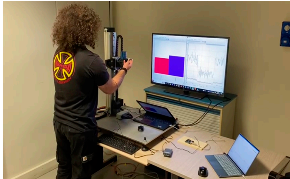
Figure 16. The tests were carried out in front of a monitor. On the dynamic bar graph, the reference signal (red bar) and the signal of the actual position (blue bar). On the right, the signals of the forces produced by the participant and the machine.
