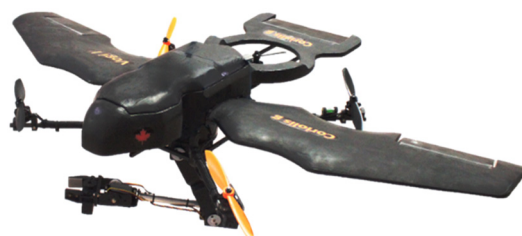
Figure 2. Pitch-decoupled VTOL UAV with a robotic arm.
