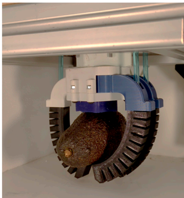
Figure 18. Example of successful grasping of an object (avocado).
