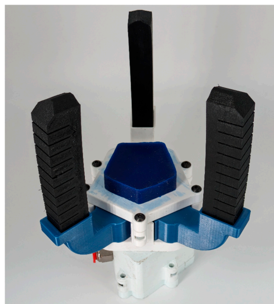
Figure 9. The developed gripper composed of soft silicone palm, TPU actuators, and a PLA structure.
