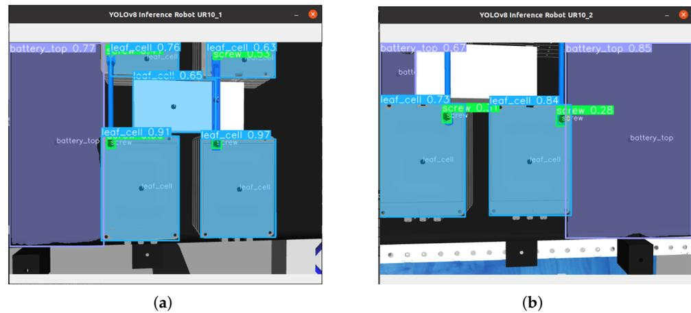
**Figure 11.** YOLOv8 output results taken from two different cameras in the simulation environment. (a) The result of the image taken from the camera attached to UR10\_1; (b) the result of the image taken from the camera attached to UR10\_2.
