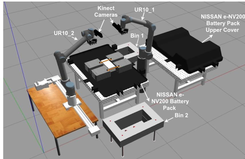
**Figure 5.** An illustration of the simulation environment with a battery pack and two UR10 robots with vacuum grippers and depth cameras attached to the end-effectors.
