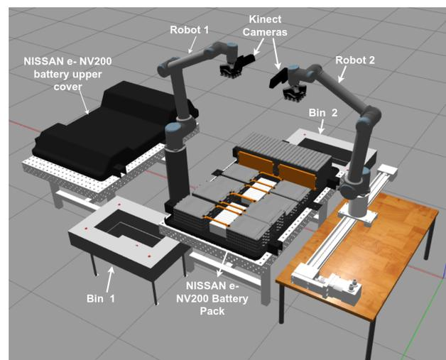
**Figure 3.** An illustration of the simulation environment with a battery pack and two UR10 robots with vacuum grippers and Kinect cameras attached to the end-effectors.
