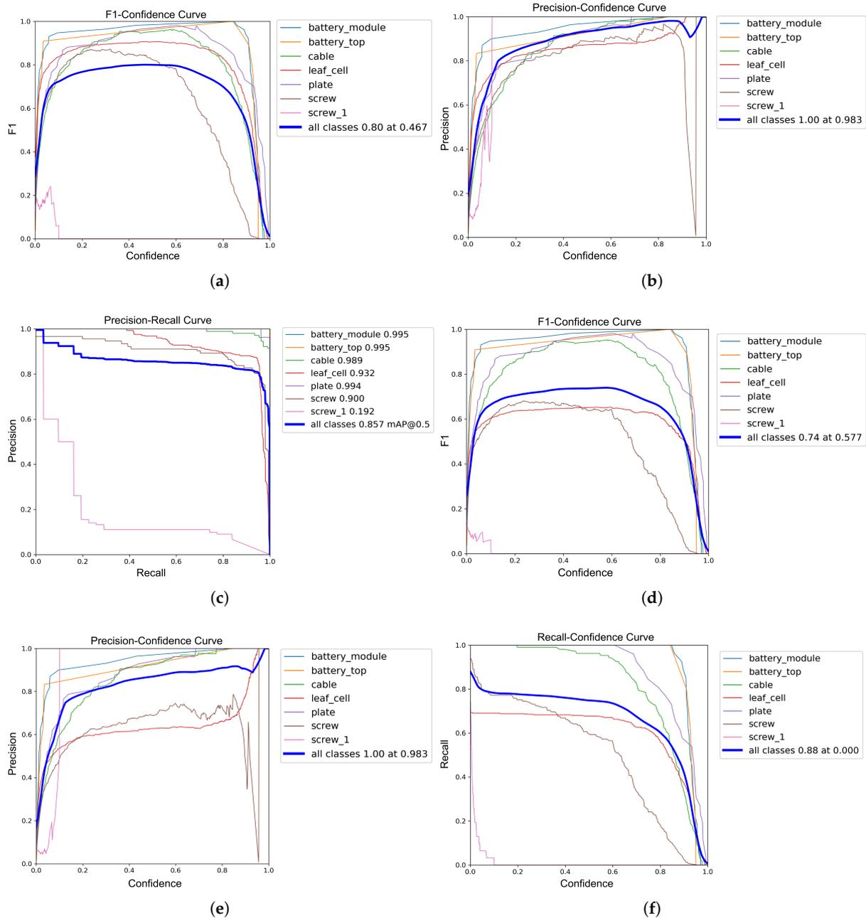
**Figure 10.** Performance metrics of the trained model. (a) BoxF1 Curve. (b) BoxP Curve. (c) BoxPR Curve. (d) MaskF1 Curve. (e) MaskP Curve. (f) MaskR Curve.
