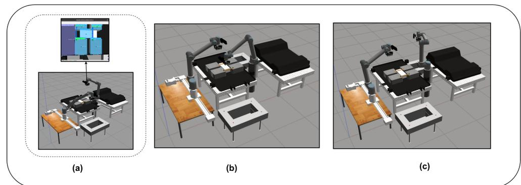
**Figure 9.** Removing the screw with UR10\_1. (a) The object labelled screw is detected by the vision algorithm. (b) The UR10\_1 robot picks up the detected object and (c) places the object at the targeted point.
