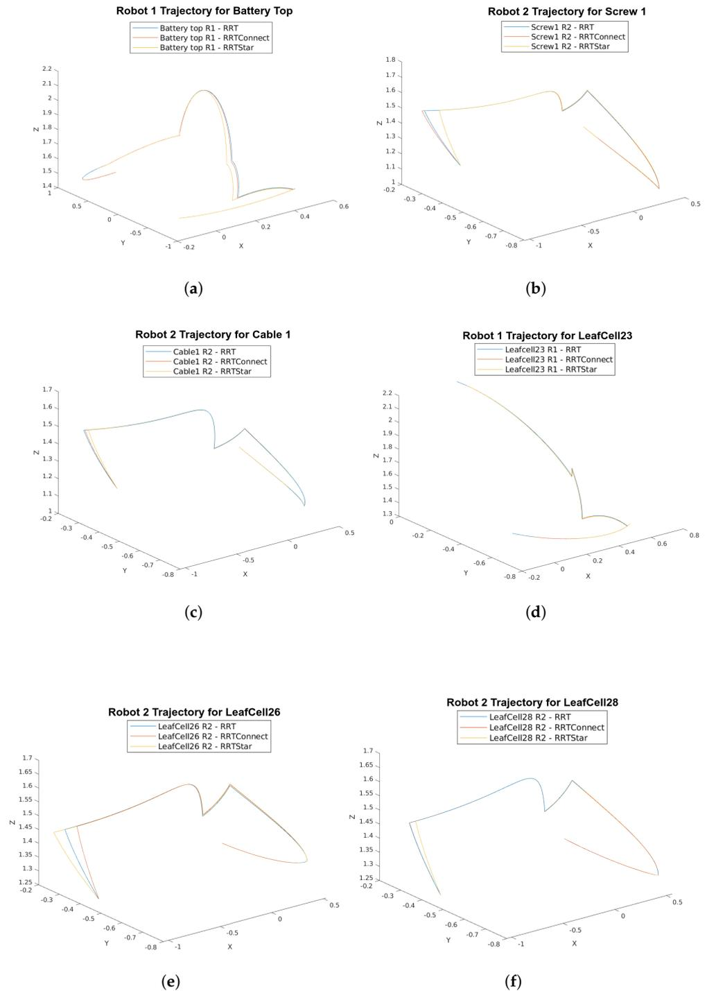
**Figure 12.** Trajectory graphs followed by robots during the disassembly process of randomly selected objects using the RRT, RRTConnect, and RRTStar planners. (a–f) Trajectories followed by robots during the disassembly of objects called battery\_top, screw1, cable1, leafcell23, leafcell26, and leafcell28, respectively.
