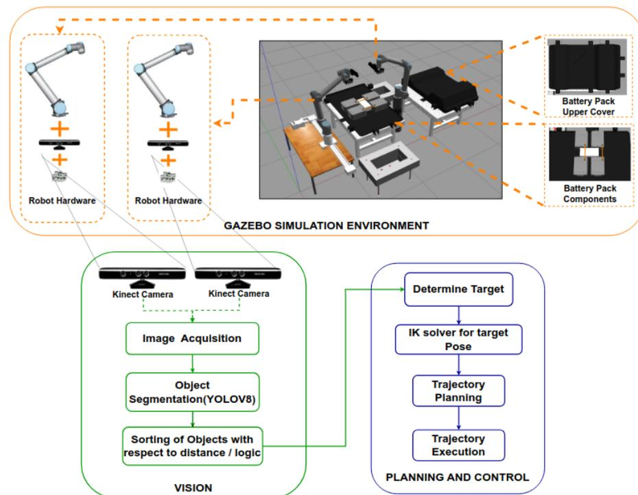
**Figure 2.** A graphical overview of the task planner designed in the simulation environment, the proposed vision algorithm, and the planning and control algorithm.
