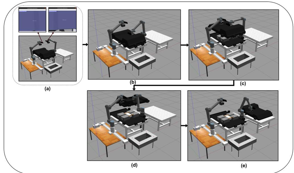
**Figure 7.** Removing the battery pack top cover with UR10\_1. (a) The object labelled battery\_top is detected by the vision algorithm. (b) The UR10\_1 robot moves to remove the detected object, (c) picks up the object, (d) moves the object to the drop location, and (e) places the object at the targeted point.
