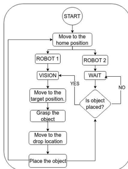
Figure 4. Developed task planner flowchart.
