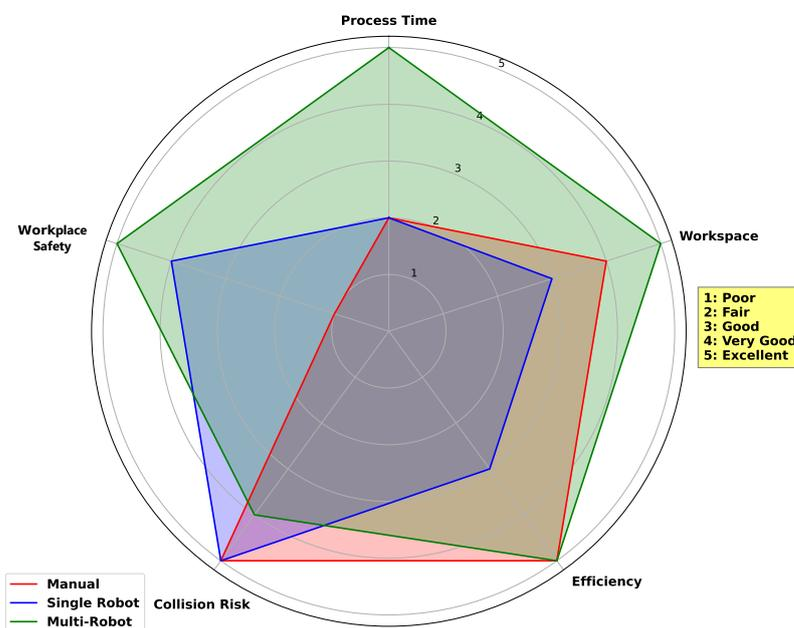
**Figure 1.** A visual comparison of three disassembly methods—manual, single-robot, and multi-robot—across five critical operational aspects: process time, workspace, efficiency, collision risk, and workplace safety. Each aspect is quantitatively rated on a scale from 1 to 5, where 1 indicates the least favourable outcome and 5 indicates the most favourable.
