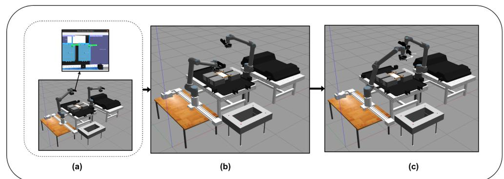
**Figure 8.** Removing the screw with UR10\_2. (a) The object labelled screw is detected by the vision algorithm. (b) The UR10\_2 robot picks up the detected object and (c) places the object at the targeted point.
