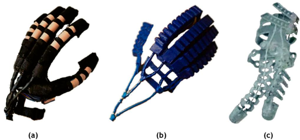
**Figure 4.** Variations in soft glove designs: (a) fluidic bladder-based, (b) digital manufacturing-derived, and (c) polymer structural component-based models.
