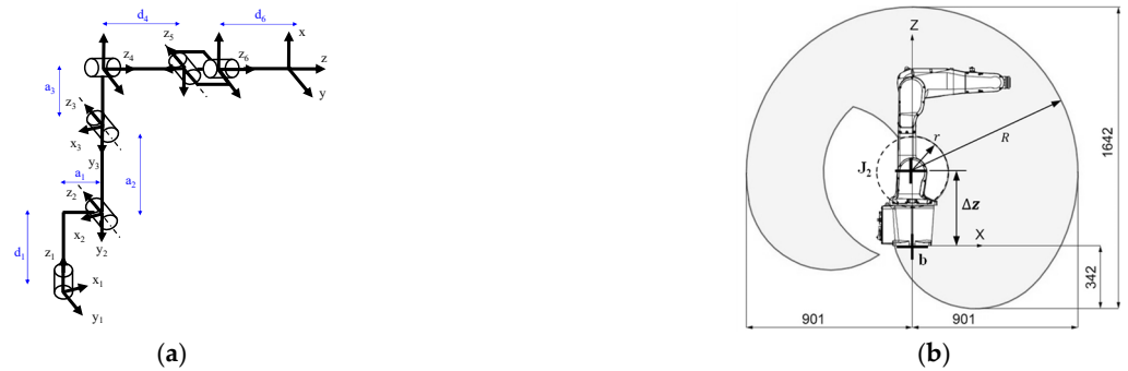
Figure 1. The 6-DOF robot representation: serial-linked revolute joints (a); preliminary reachability of the ABB IRB1200-5/0.9 robot for reference (b).
