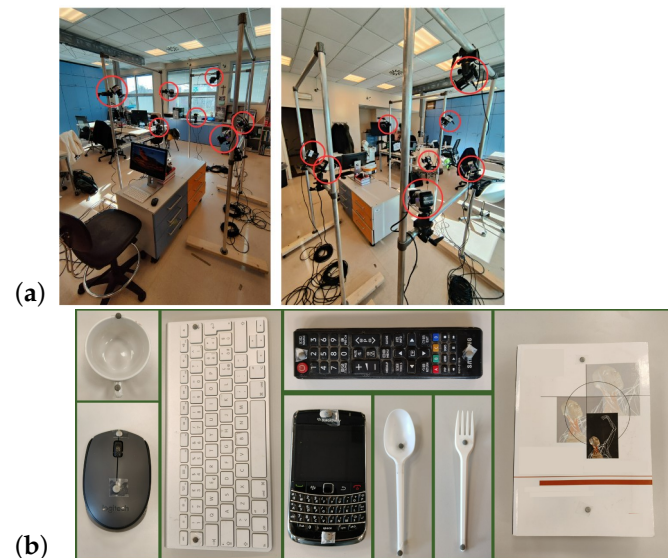
Figure 4. Experimental setup for Control Validation phase; VERO v2.2 cameras are shown in red circles (a). Objects used in the second session of the experimental protocol (b).
