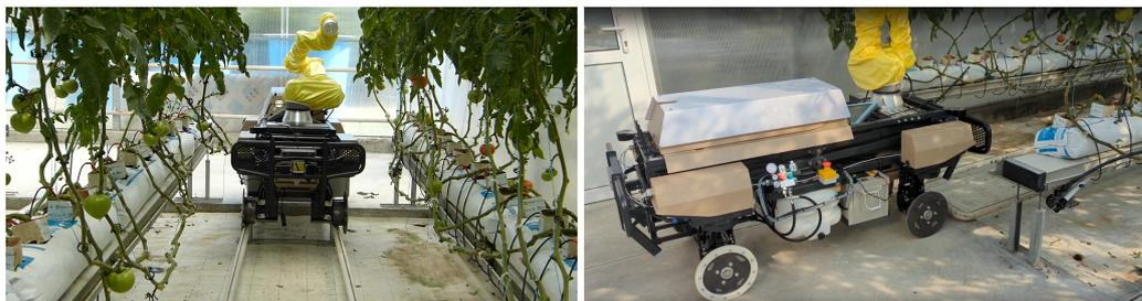
**Figure 1.** The mobile robotic platform used in the navigation pipeline. The left image displays the front side of the robot while traversing on the greenhouse’s corridor rails. LiDAR and a stereo camera are attached on this side. The right image displays the side view of the robotic platform with the biopesticide tank and the 2D laser scanners.
