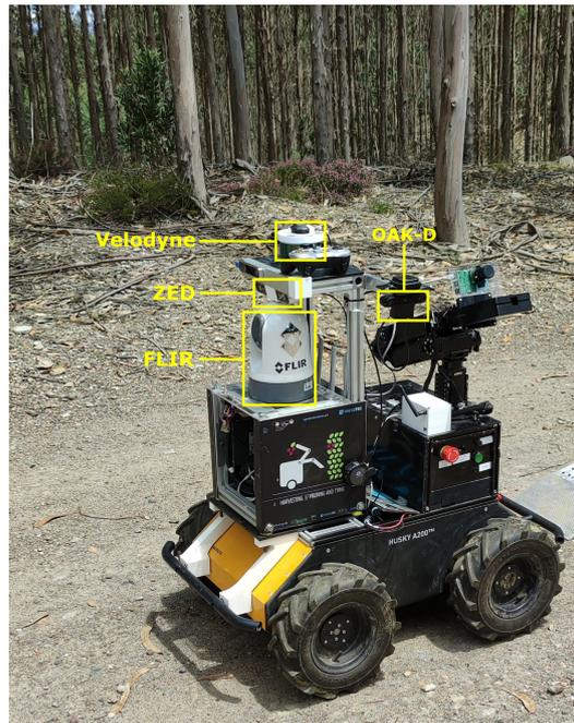
**Figure 18.** AgRob V16 mobile platform and its multisensory system for forestry perception. Reproduced from [350] with permission.
