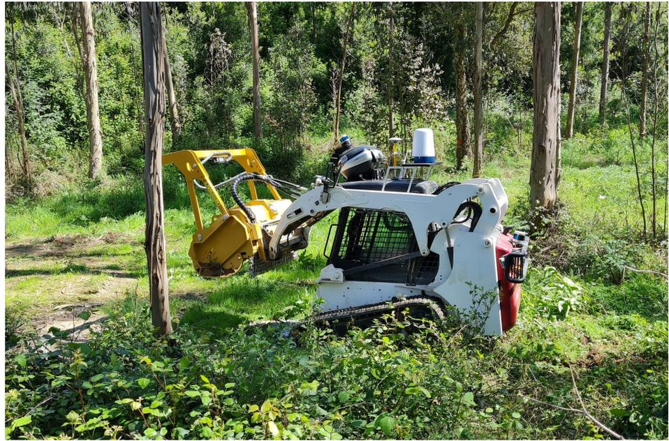
**Figure 2.** The *Ranger* landscape maintenance robot developed in the SEMFIRE project. For more details, please refer to [32].
