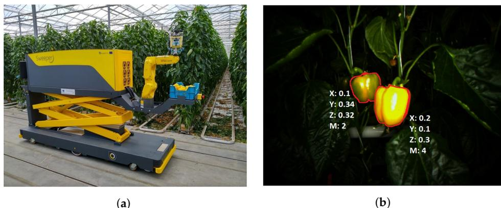
**Figure 6.** The Sweeper robot (a), a sweet-pepper harvesting robot operating in a greenhouse. (b): the output of Sweeper’s pepper detection technique. The Sweeper project aims to develop an autonomous harvesting robot, based on the developments of the CROPS project, which can operate in real-world conditions. Reproduced with permission. Source: [www.sweeper-robot.eu](http://www.sweeper-robot.eu), accessed on 30 June 2023.
