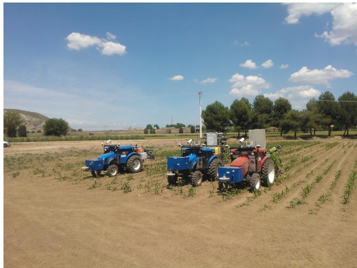
**Figure 4.** The RHEA robot fleet on a wheat spraying mission. RHEA focused on the development of novel techniques for weed management in agriculture and forestry, mainly through the usage of heterogeneous robotic teams, involving autonomous tractors and Unmanned Aerial Vehicles (UAVs). Reproduced with permission.
