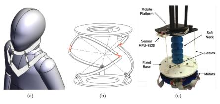
**Figure 4.** Neck joint mechanisms: (**a**) 3-RPS mechanism by Vellore Institute of Technology, redrawn based on [1]; (**b**) 3-RXS mechanism by the University of Technology Beijing [38], available under a Creative Commons Attribution License; (**c**) 3-CDPM mechanism by University Carlos III of Madrid [3], available under a Creative Commons Attribution License.
