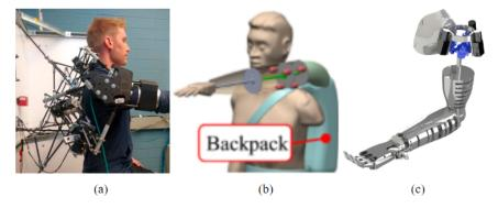
**Figure 5.** Shoulder joint mechanisms: (**a**) 4B-SPM mechanism by Arizona State University [49]; (**b**) cable-driven mechanism by Chiba University [50]; (**c**) 3-RRR mechanism by Universidad de Guanajuato [19]. All are available under a Creative Commons Attribution License.
