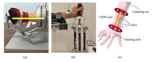
**Figure 6.** Wrist joint mechanisms: (a) 6-SPS/PS mechanism by the University of Macau [63]; (b) 3-CSPM mechanism by Kwangwoon University [69]; (c) 4-CDPS mechanism by Southeast University [77]. All are available under a Creative Commons Attribution License.
