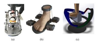
**Figure 8.** Ankle joint mechanisms: (a) 2-UPS/RRR mechanism by Beijing University [104]; (b) S-4SPS mechanism by the University of Nottingham [105]; (c) spherical mechanism by Instituto Politécnico Nacional, Mexico [109]. All are available under a Creative Commons Attribution License.
