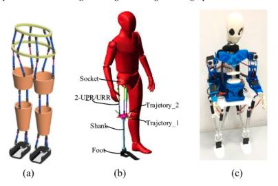
**Figure 7.** Hip joint mechanisms: (**a**) 6 SPS mechanism by Shangai University [83]; (**b**)4 RPS mechanism by Jiaotong University [84]; (**c**)3UPR mechanism by the University of Cassino and Southern Latium [87]. All are available under a Creative Commons Attribution License.
