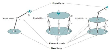
Figure 3. Architectural design of serial, parallel, and hybrid robots.
