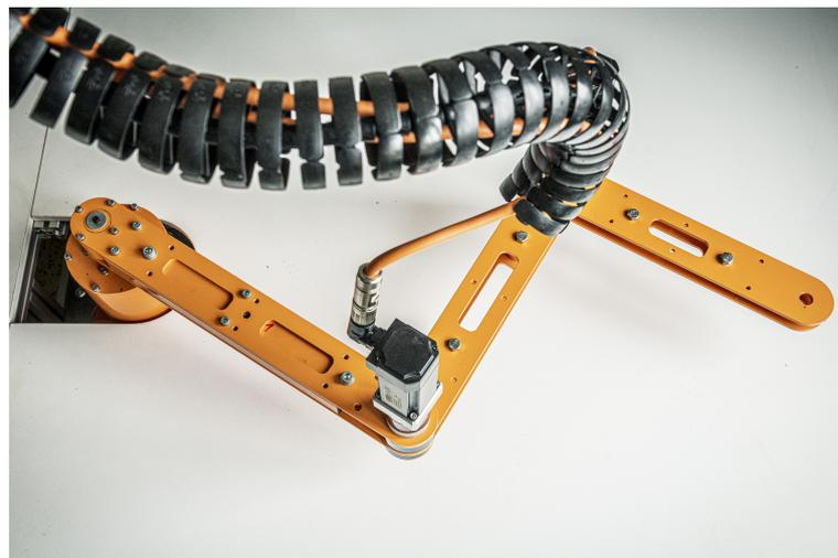
**Figure 6.** Experimental model of the printing robot.
