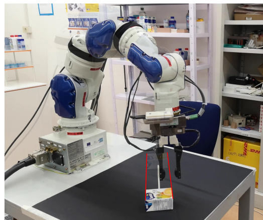
Figure 7. Setup of the first experiment: testing of the MPC pushing controller.
