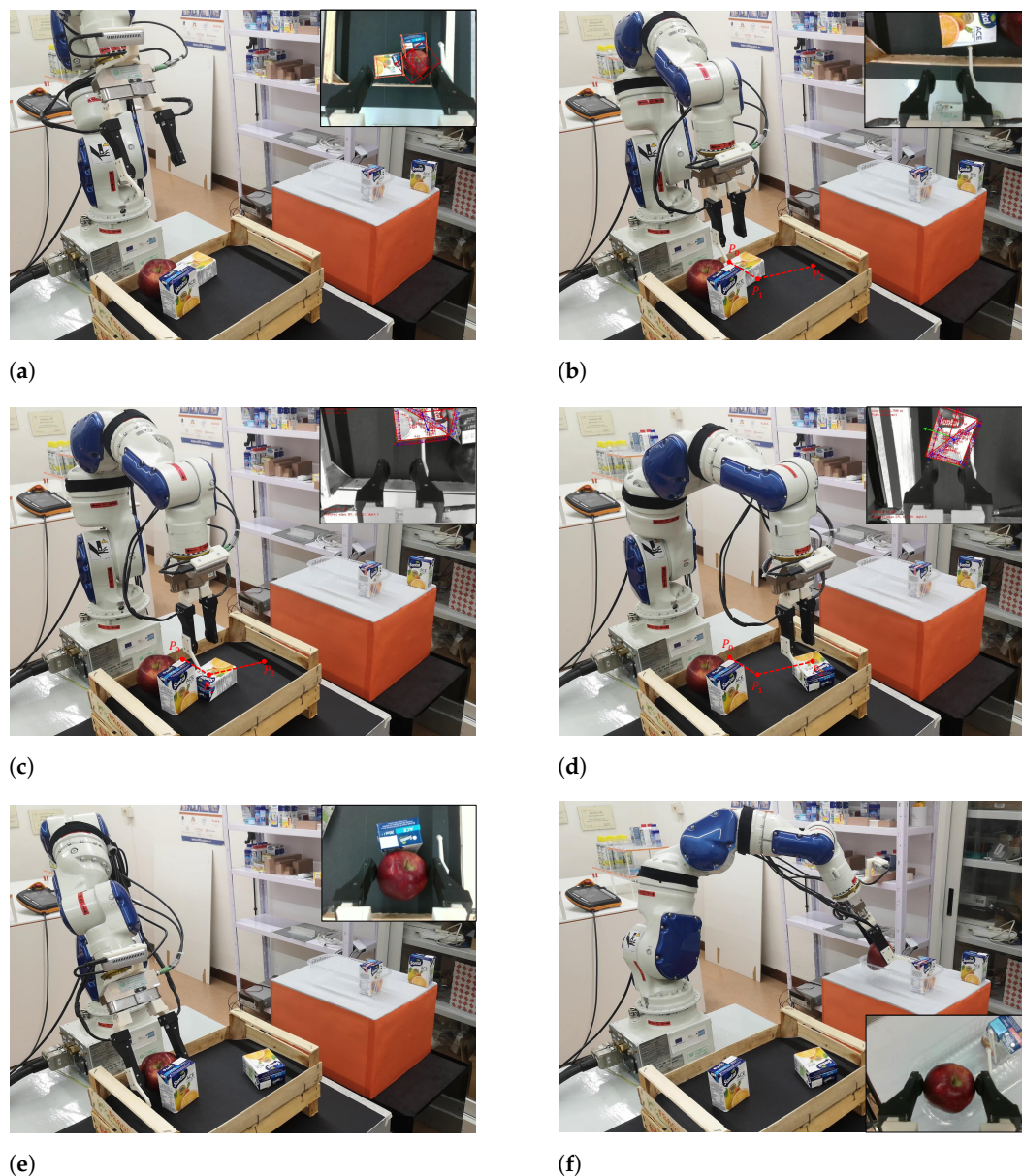
Figure 16. Screenshots of the experiment execution. (a) Initial scene to pick the red apple. The grasp is unfeasible due to the obstacles in the scene. (b) The robot moves to the pre-push pose to execute the pushing maneuver. (c) The robot reaches the first point P_1 of the desired trajectory. The picture-in-picture image shows the camera view used by the tracking system. (d) The robot reaches the second point P_2 of the desired trajectory. The picture-in-picture image shows the camera view used by the tracking system. (e) The robot is now able to grasp the red apple in the box. The picture-in-picture image is the camera view. (f) The robot places the red apple in the desired container.
