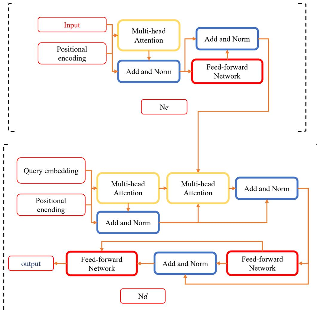
**Figure 3.** The transformer model.
