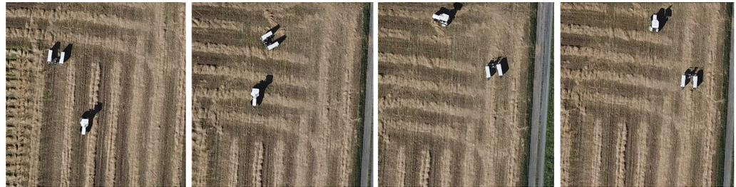
**Figure 9.** An aerial imagery of the leader–follower navigation inside the field. The sequences illustrate how the robot followed the tractor during a U-turn.
