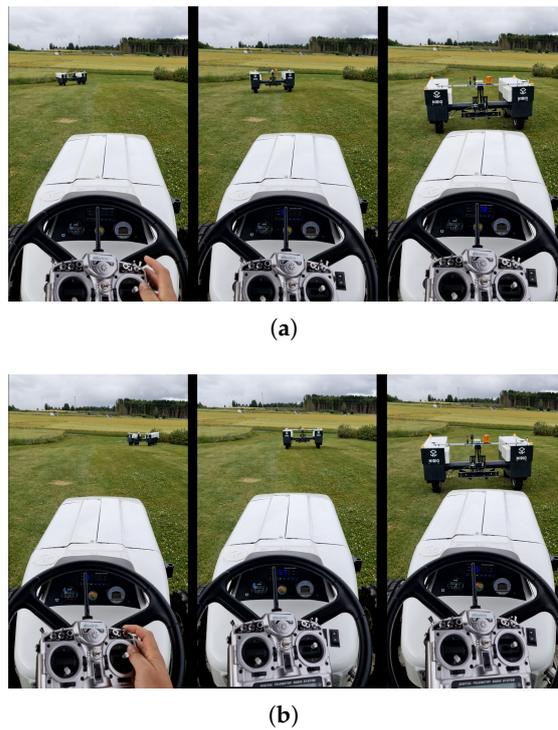
**Figure 6.** The evolution of both the distance and orientation separating the robot from the tractor during the static waypoint experiments. The robot stopped at 6.2 m and 5.7 m, respectively, when beginning the navigation from the two starting positions. (a) Static waypoint navigation: starting position 1. (b) Static waypoint navigation: starting position 2.
