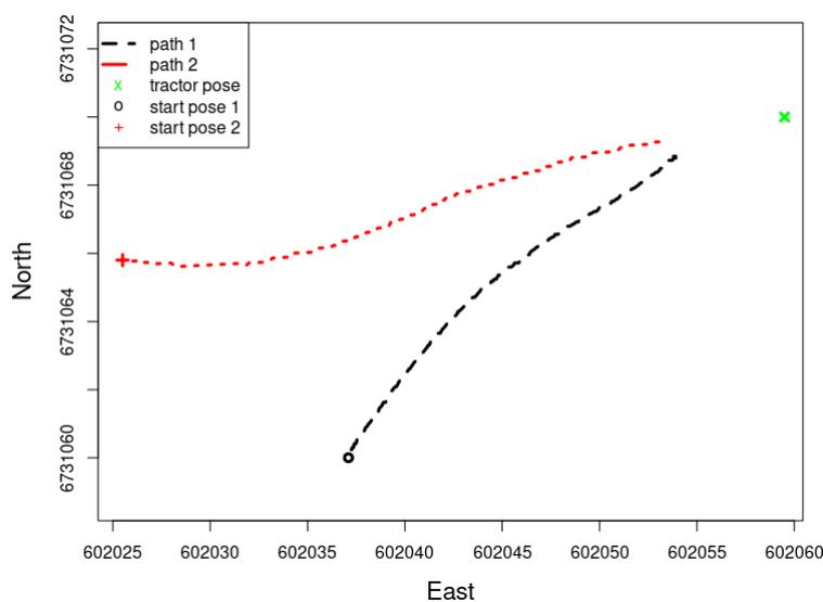
**Figure 7.** The recorded GNSS trajectory of the robot during the tuning of the controller gains. The black trajectory (long dashed line) represents the path that the robot followed starting from “start pose 1”. The red trajectory (short dashed line) represents the path that the robot followed starting from “start pose 2”. The green “x” represents the fixed location of the tractor.
