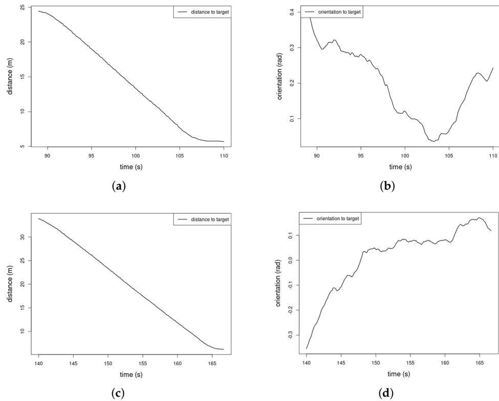
**Figure 8.** The evolution over time of both the distance and orientation separating the robot from the tractor during the static waypoint experiments. The robot stopped at 6.2 m and 5.7 m, respectively, when beginning its navigation from the two starting positions. (a) Distance: start pose 1. (b) Orientation: start pose 1. (c) Distance: start pose 2. (d) Orientation: start pose 2.
