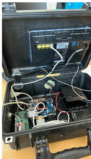
**Figure 2.** The equipment installed on the tractor: The Jetson AGX Xavier, the Piksi-multi GNSS-RTK board, and the wireless router. The IMU and the GNSS receiver are mounted on the chassis of the tractor.
