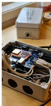
**Figure 4.** The dual GNSS-RTK receivers added to the robot for a robust heading estimation
