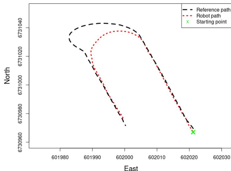
**Figure 10.** The path of the robot and its reference point to the tractor.
