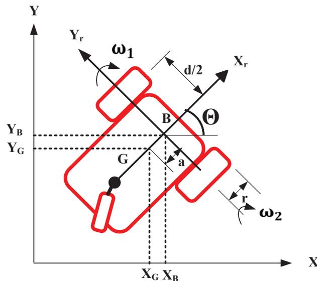
Figure 3. Kinematic model of the differential-drive mobile robot.
