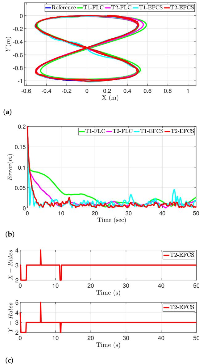
**Figure 5.** Performance of the proposed system in the face of measurement noise. (a) Desired vs. actual positions of the robot path in the face of sensor noise. (b) Distance error evolution for different controllers in the face of measurement noise. (c) Evolution of the fuzzy rules for T2-EFCS in the face of measurement noise.
