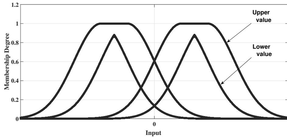
Figure 1. Interval type-2 Gaussian membership function.
