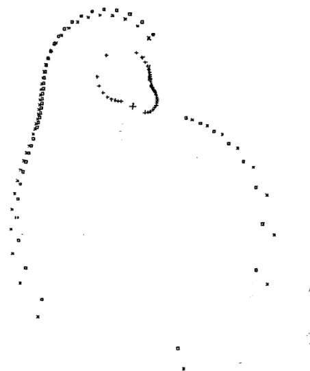
Figure 16. The three Burmester curves for a triad in six precision positions. There are two circle-point curves (corresponding to the two moving pivots) and one center-point curve [21] (p. 86).
