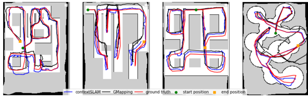
Figure 7. Predicted trajectories of contextSLAM (blue) and GMapping (black) in the four environments with respect to the ground truth (red).
