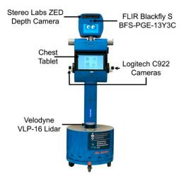
Figure 4. Blueberry Robot with labeled robot components.
