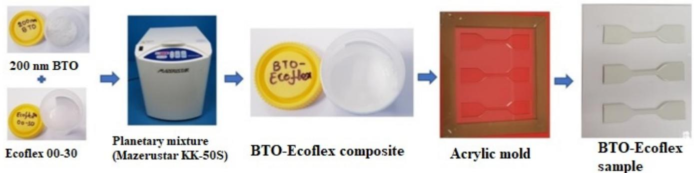
**Figure 2.** BTO-Ecoflex<sup>TM</sup> composite preparation process.
