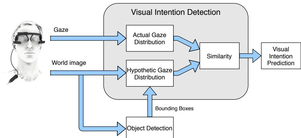
**Figure 3.** The block diagram of the GazeEMD system.
