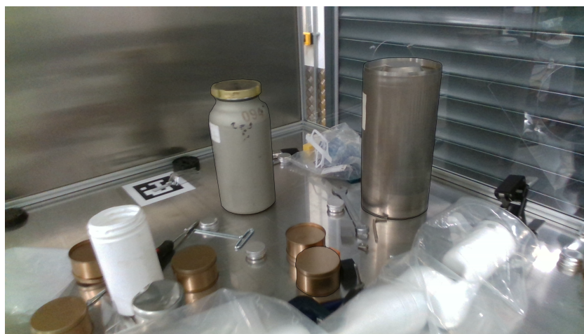
Figure 1. The glovebox mock-up and the manipulation system with representative cylindrical containers to store radioactive substances.
