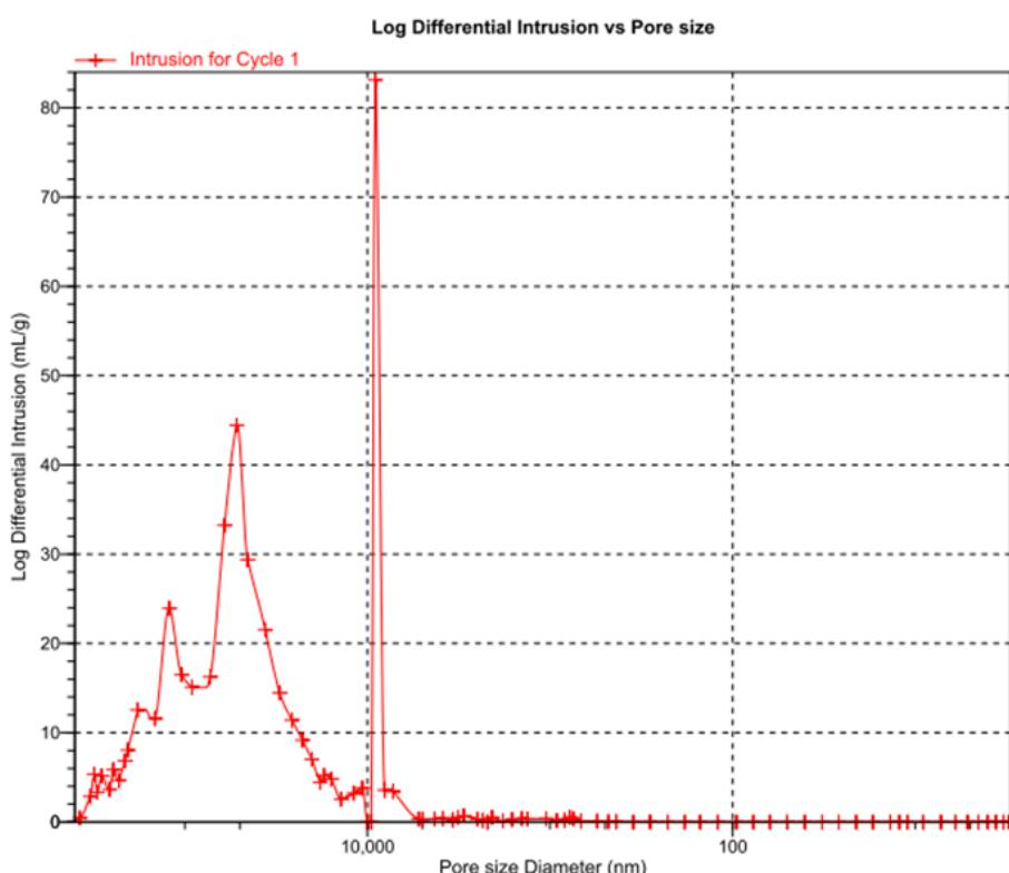
**Figure S1. Mercury porosimetry report of HLC scaffold.** The porosity of the HLC scaffold was over 99%.
