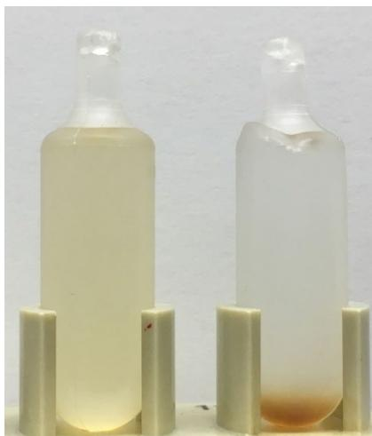
**Figure S1.** Photograph of one of the nanoparticle formulations before (left) and after (right) centrifugation at  $4.3 \times 10^5$  g for 1 h.
