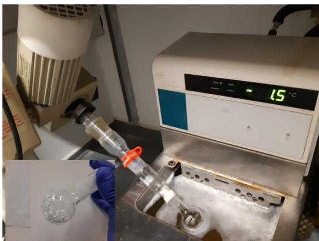
**Figure 2.** Ice-shell purification using a 10 mL round bottom flask.
