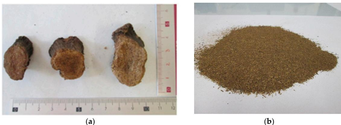
**Figure 1.** Samples of raw banana rachis (a) and rachis powder after grinding and drying (b).
