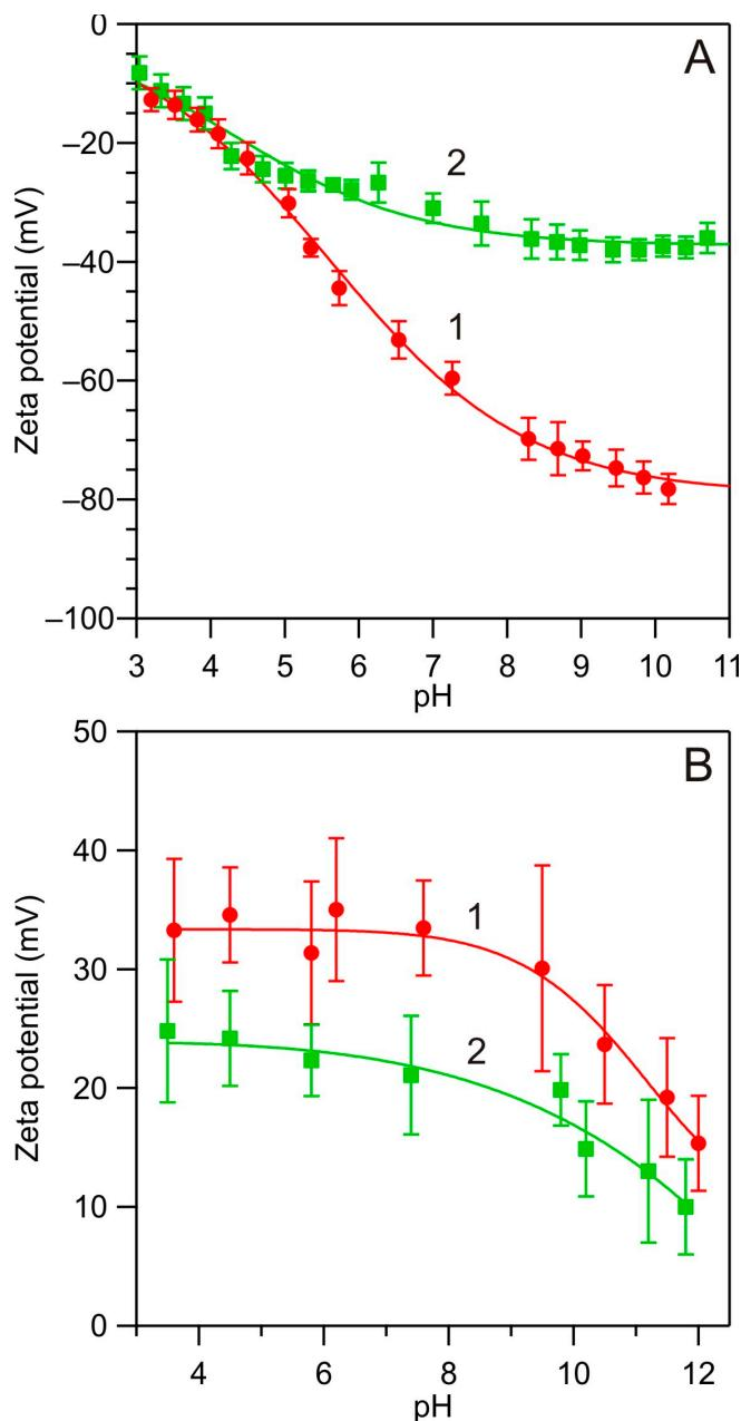
**Figure 3.** (A) Zeta potential of the bare silica substrate vs. pH determined by streaming current measurements: (1) 10 mM NaCl and (2) 150 mM NaCl. (B) Zeta potential of the PARG-covered silica substrate vs. pH determined by streaming potential measurements (microfluidic cell): (1) 10 mM NaCl and (2) 150 mM NaCl. The lines are a guide for the eyes.
