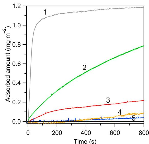
**Figure 7.** Kinetics of HSA adsorption on bare silica sensor determined by reflectometry for various pHs, albumin bulk concentration  $c_b = 5 \text{ mg L}^{-1}$ ,  $Q = 8.33 \times 10^{-3} \text{ cm}^3 \text{ s}^{-1}$ , 150 mM NaCl: (1) pH 4.0, (2) pH 4.8, (3) pH 5.4, (4) pH 7.4, and (5) pH 8.6.
