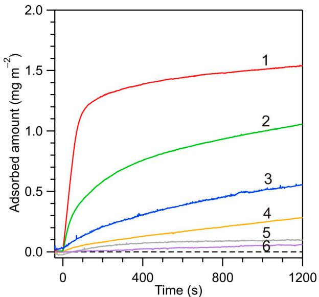
**Figure 8.** Kinetics of HSA adsorption on PARG-covered silica sensor determined by reflectometry for various pHs, albumin bulk concentration  $c_b = 5 \text{ mg L}^{-1}$ , 150 mM NaCl,  $Q = 8.33 \times 10^{-3} \text{ cm}^3 \text{ s}^{-1}$ : (1) pH 7.4 (NaCl), (2) pH 8.6, (3) pH 7.4 (PBS); (4) pH 5.8; (5) pH 4.0, and (6) pH 3.5.
