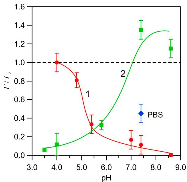
**Figure 9.** Dependence of the plateau coverages of HSA (normalized to the maximum coverage of  $1.1 \text{ mg m}^{-2}$  for the bare silica) for 150 mM NaCl on pH: (1) adsorption on bare silica sensor and (2) adsorption on PARG-covered sensor. The blue point presents experimental data for PBS solution. The lines are guides for the eyes.
