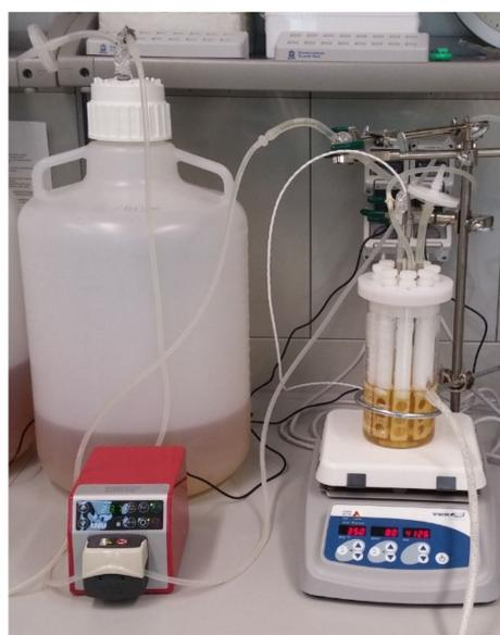
Figure 8. CDC biofilm reactor (BioSurface Technologies, Bozeman, MT, USA).
