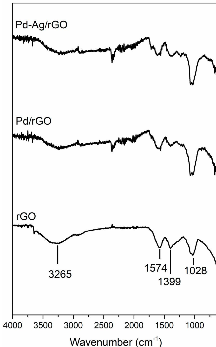
**Figure 3.** Fourier Transform Infrared (FTIR) spectra of fabricated GO, Pd/rGO, and Pd-Ag/rGO nanostructures using stevia leaf extract.
