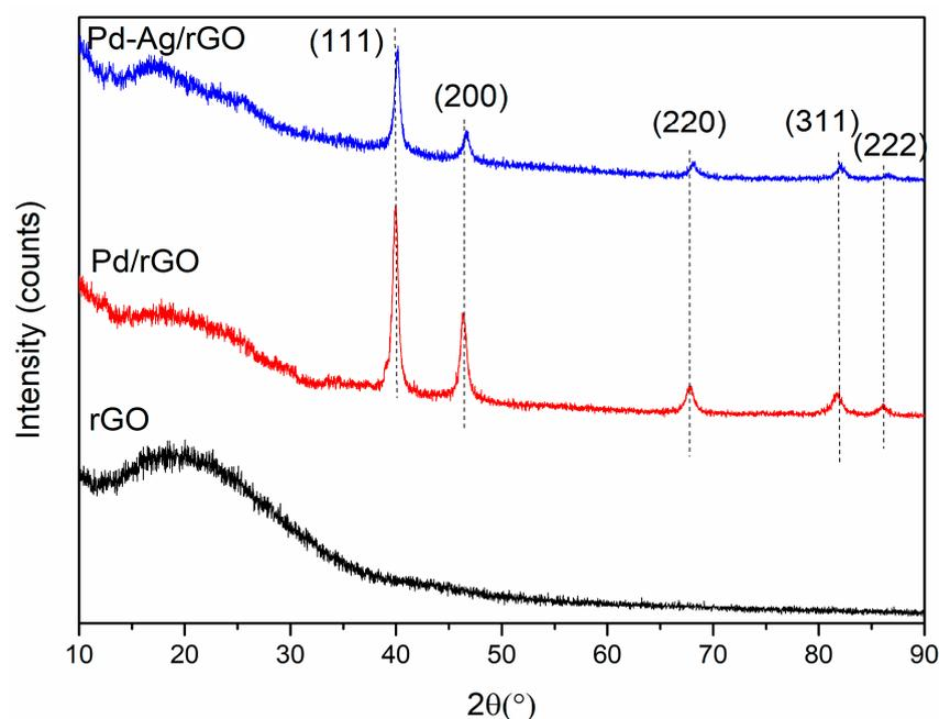
**Figure 2.** X-ray diffraction results of synthesized materials of rGO, Pd/rGO, and Pd-Ag/rGO nanostructures.
