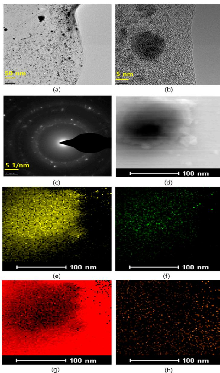
**Figure 4.** Different magnification TEM images of Pd-Ag nanoparticles anchored on reduced graphene oxide sheets (a) 50 nm (b) 5 nm (c) Selected Area Electron Diffraction (SAED) pattern (d) STEM-HAADF image and elemental mapping of (e) palladium (f) silver, (g) carbon and (h) oxygen elements presence in Pd-Ag/RGO nanostructures.
