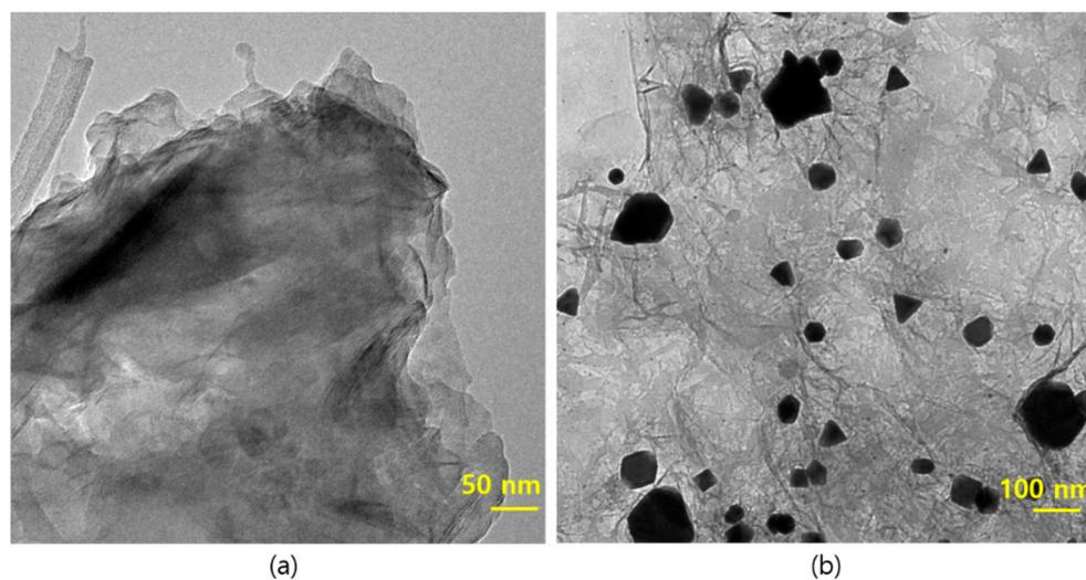
**Figure 5.** TEM images of Pd/rGO and rGO nanostructures. (a) rGO nanosheets, and (b) Pd nanostructures anchored on rGO nanosheets.
