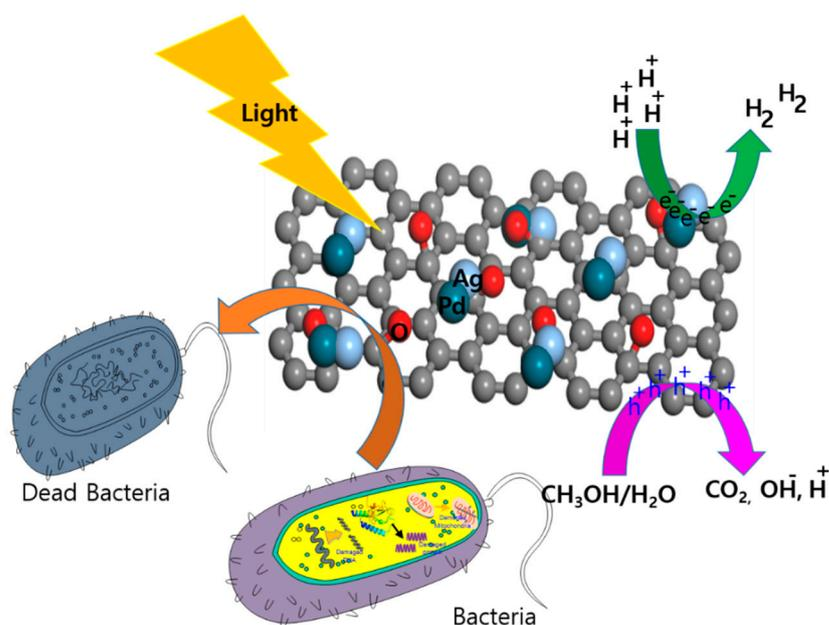
**Figure 8.** Schematic representation of photocatalytic  $H_2$  production and hypothetical antimicrobial mechanism of prepared catalysts.
