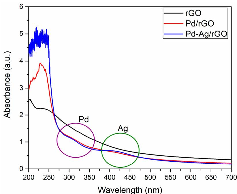
**Figure 1.** UV-Vis absorption spectra of prepared rGO, Pd/rGO, and Pd-Ag/rGO nanostructures using plant leaf extract.
