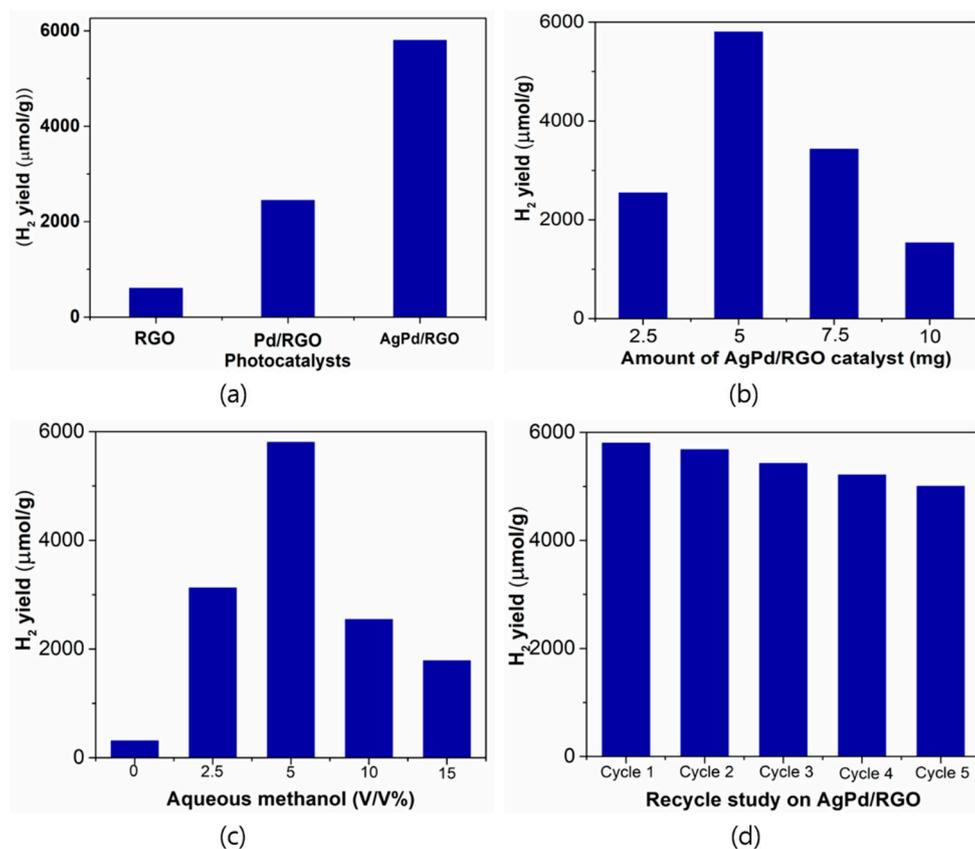
**Figure 7.** (a) Photocatalytic H<sub>2</sub> production with prepared catalysts (b) Different amounts of Pd-Ag/rGO catalyst for H<sub>2</sub> production (c) Different amounts of sacrificial agent (methanol) for H<sub>2</sub> production (d) Reusability test for H<sub>2</sub> production using Pd-Ag/rGO photocatalyst.
