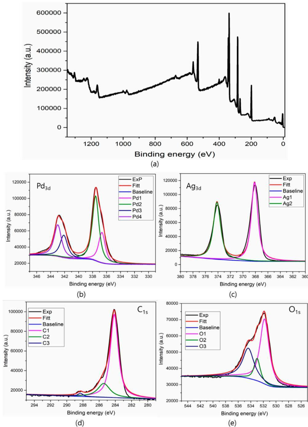
**Figure 6.** XPS spectra of Pd-Ag/RGO nanostructures (a) survey scan (b) Palladium (c) Silver (d) Carbon and (e) Oxygen.
