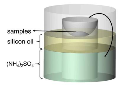
Figure S6. The schematic device for crystallisation with silicon oil floating on the reservoir buffer. The silicon oil (yellow) floating on the reservoir buffer formed a barrier to slow down the water vapour diffusion speed from the sample drop to the absorbing (NH<sub>4</sub>)<sub>2</sub>SO<sub>4</sub> buffer.
