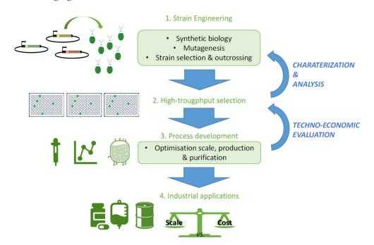
Figure 3. The key steps in bioengineered green algae production (adapted from Scranton et al. [69]).
