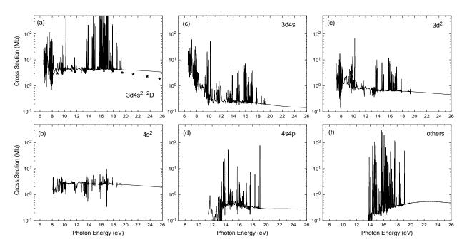
**Figure 1.** Cross sections for photoionization of the ground  $3d4s^2$   $^2D$  state of Sc. (a) total cross-sections from the present BSR-81 model are compared with the MBPT calculations of Altun & Manson [14] (asterisks). (b–e) show summed partial cross-sections for leaving the residual Sc<sup>+</sup> ion in the final states of the  $4s^2$ , 3d4s, 4s4p, and  $3d^2$  configurations, respectively, along with contribution of all other channels in (f).
