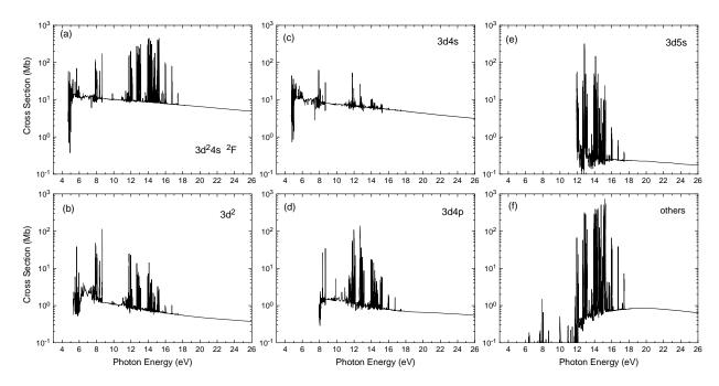
**Figure 2.** Cross sections for photoionization from the excited  $3d^24s$   $^2F$  state of Sc. (a) total cross-sections from the present BSR-81 model and (b–f) show summed partial cross-sections for leaving the residual Sc<sup>+</sup> ion in the final states of the  $3d^2$ , 3d4s, 3d4p, and 3d5s configurations, respectively, along with contributions of all other channels.
