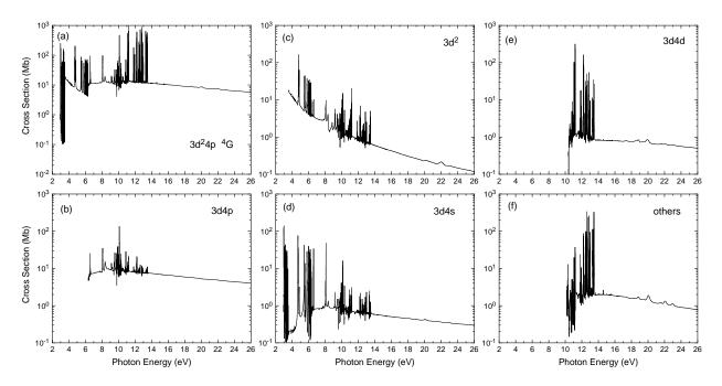
**Figure 4.** Photoionization cross-sections from the excited  $3d^24p^4G$  state of Sc. (a) shows total cross-sections from the present BSR-81 model whereas (**b**-**f**) show summed partial cross-sections for leaving the residual Sc<sup>+</sup> ion in the final states of the 3d4p,  $3d^2$ , 3d4s, and 3d4d configurations, respectively, along with the contribution of all other channels.
