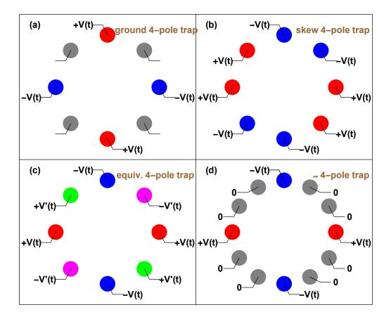
leads to a pure quadrupole trap with the additional grounded electrodes ensuring the points of zero potential, thereby providing additional stability against stray fields.
