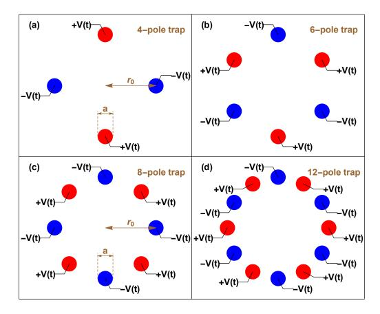
**Figure 1.** Electrode potential configuration for normal operation of (**a**) a 4-pole trap, (**b**) a 6-pole trap, (**c**) an 8-pole trap and (**d**) a 12-pole trap, where  $V(t) = V_0 \sin \omega t$ . We keep the parameters  $r_0$  and *a* fixed for all the trap configurations. Note that the 12-pole trap in (**d**) is also equivalent to the superposition of three quadrupole traps  $(e_1, e_4, e_7, e_{10}), (e_2, e_5, e_8, e_{11})$  and  $(e_3, e_6, e_9, e_{12})$ .
