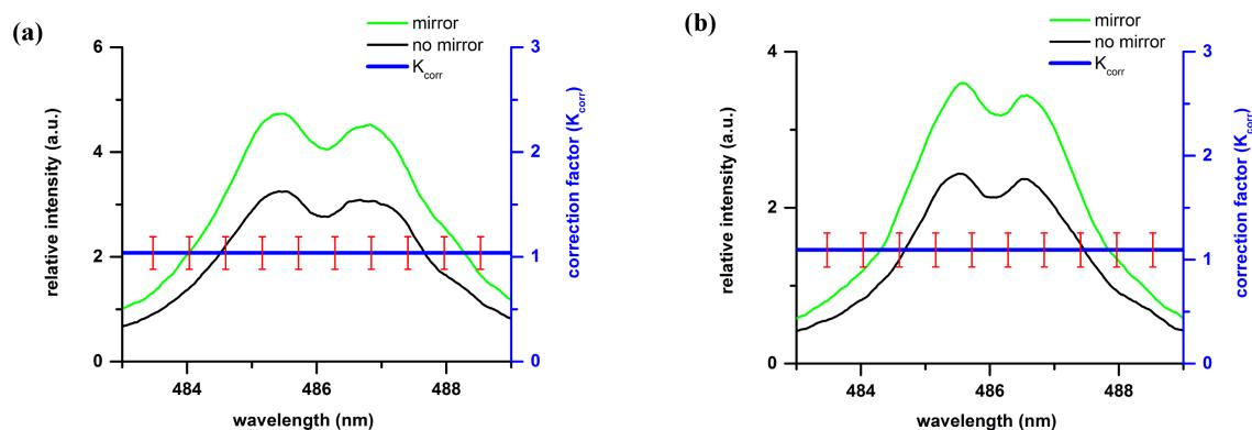
**Figure 12.** Measured, Savitzky–Golay filtered  $H_{\beta}$  air-plasma data with and without using a doubling mirror [33]. The correction factor,  $K_{\text{corr}}$ , is almost equal to 1. The error bars indicate the estimated errors in determination of the correction factor. Time delay: (a)  $5 \mu\text{s}$ ; and (b)  $7 \mu\text{s}$ .
