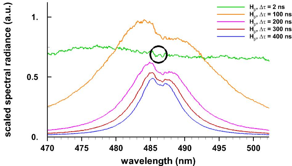
**Figure 6.** Line shapes of  $H_{\beta}$  for the indicated time delays. The encircled area in the 2-ns time-delay data shows  $H_{\beta}$  absorption, in other words,  $H_{\beta}$  laser-plasma self-absorption.
