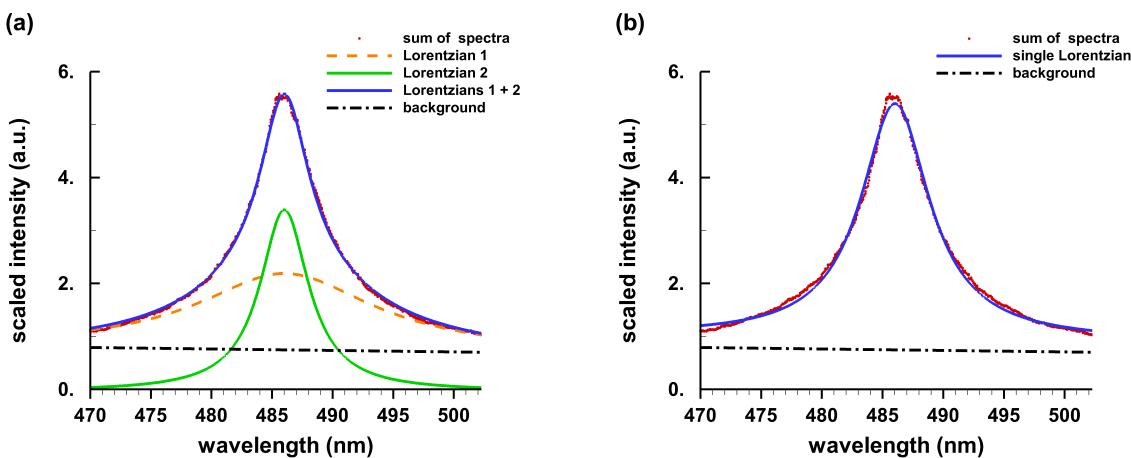
**Figure 7.** Fitting to summed  $H_{\beta}$  profiles. (a) Two Lorentzians of 4.9 and 17.6-nm widths indicating electron densities of 1.1 and  $5.8 \times 10^{17} \text{ cm}^{-3}$ , respectively. (b) Single Lorentzian fit of 6.9-nm width and  $N_e = 1.8 \times 10^{17} \text{ cm}^{-3}$ , but with discrepancies near the wings and at center.
