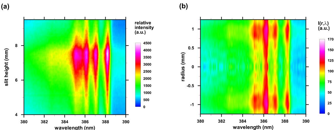
**Figure 13.** Diatomic molecular spectra: time delay 700 ns, gate width 125 ns. (a) Line-of-sight contour map of measured spectra. (b) Abel inverted spectra versus radius. Near 1 mm, the CN  $\Delta v = 0$  sequence shows 0-0, 1-1, 2-2, 3-3 and 4-4 band heads, and the second order, 193.08-nm atomic carbon line masks the 2-2 band. The CN signals are smaller near center. The carbon line appears narrower at the center than at the 1-mm radial position, indicating lower electron density at center.
