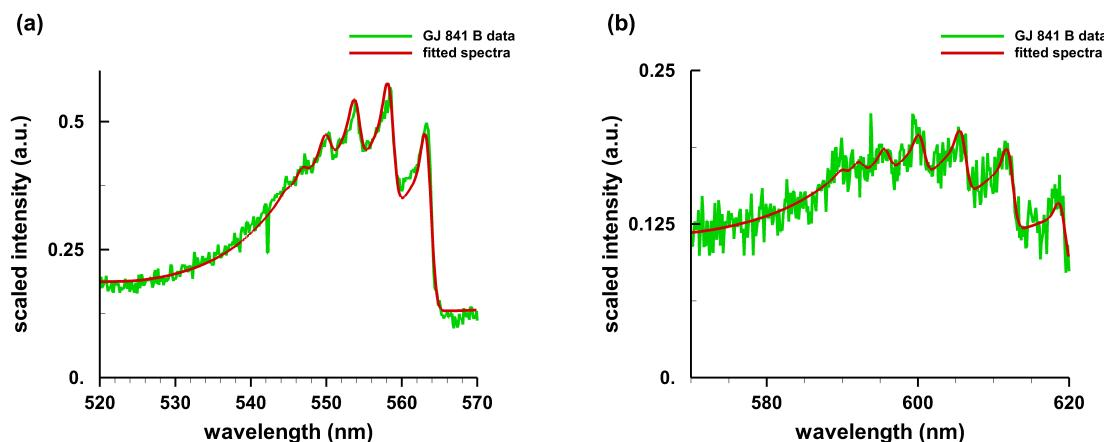
**Figure 17.** Inverted and fitted spectra for: (a)  $\Delta v = -1$  bands yielding  $T = 4.5 \text{ kK}$ ; and (b)  $\Delta v = -2$  bands indicating  $T = 4.2 \text{ kK}$ . The fitted spectral resolution equals  $\delta\lambda = 1.5 \text{ nm}$  for the spectra in (a,b).
