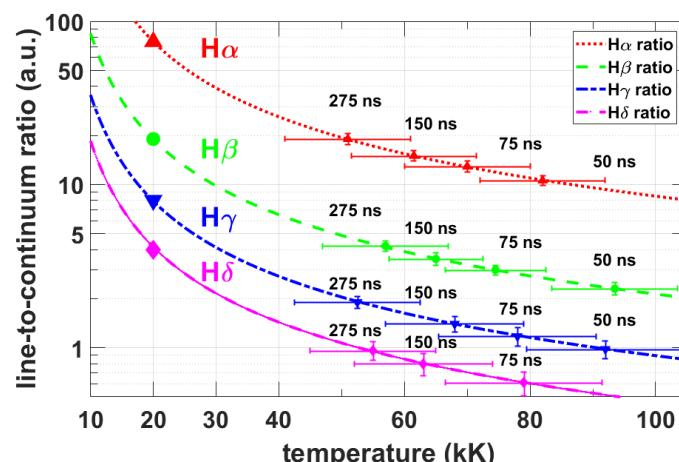
**Figure 4.** Computed and measured line-to-continuum ratios for selected time delays. Computed ratios of 75, 19, 8, and 4 are highlighted for  $H_\alpha$ ,  $H_\beta$ ,  $H_\gamma$ , and  $H_\delta$ , respectively, at 20 kK.
