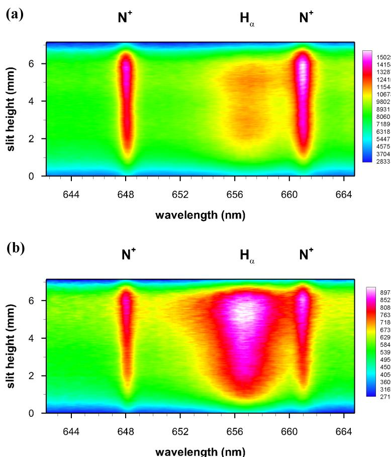
**Figure 8.** Time delay of: (a) 300 ns; and (b) 400 ns. The  $N^+$  lines allow one to determine electron density and evaluate  $H_{\beta}$  self-absorption. Reproduced from Ref. [31] with permission.
