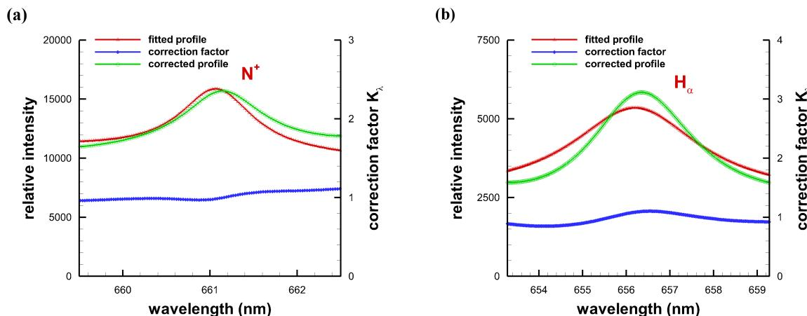
**Figure 11.** Corrected and fitted profile with correction factor. The fitted profile is obtained by determining the Lorentz profile from the experimental data: (a)  $N^+$  for a time delay of 300 ns; and (b)  $H_{\alpha}$  for a time delay of 800 ns. Slit height: 6.15 mm. Reproduced from Ref. [31] with permission.
