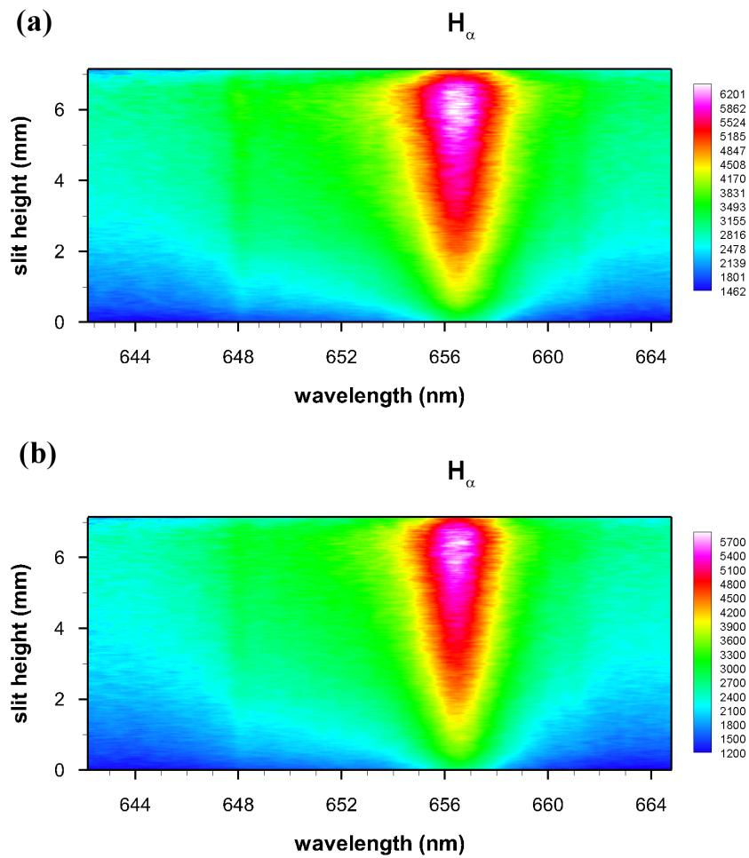
**Figure 9.** Time delay: (a) 700 ns; and (b) 800 ns. The nitrogen lines are hardly discernible in the expanding micro-plasma. Reproduced from Ref. [31] with permission.
