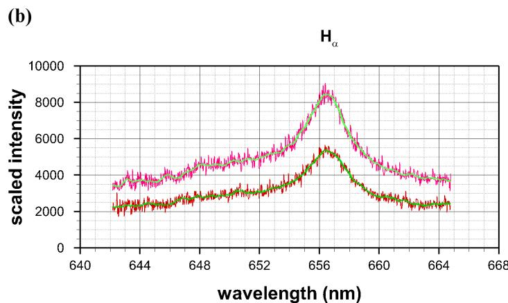
**Figure 10.** Comparison of spectra with and without mirror: (a) for 300 ns time delay; and (b) for 800 ns time delay. Slit height: 6.15 mm. Reproduced from Ref. [31] with permission.
