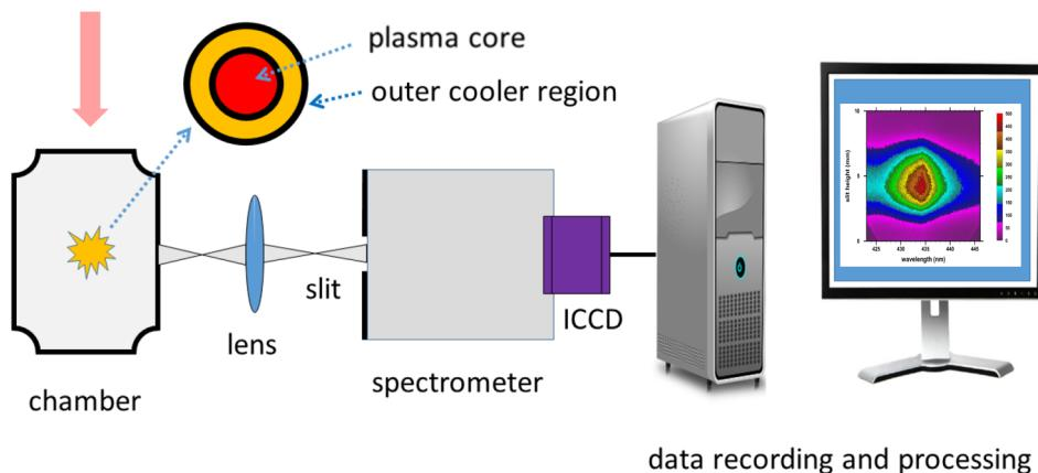
**Figure 1.** Optical breakdown plasma is generated by focusing the laser beam from the top and parallel to the slit. Time-resolved 1:1 images are recorded with the ICCD.
