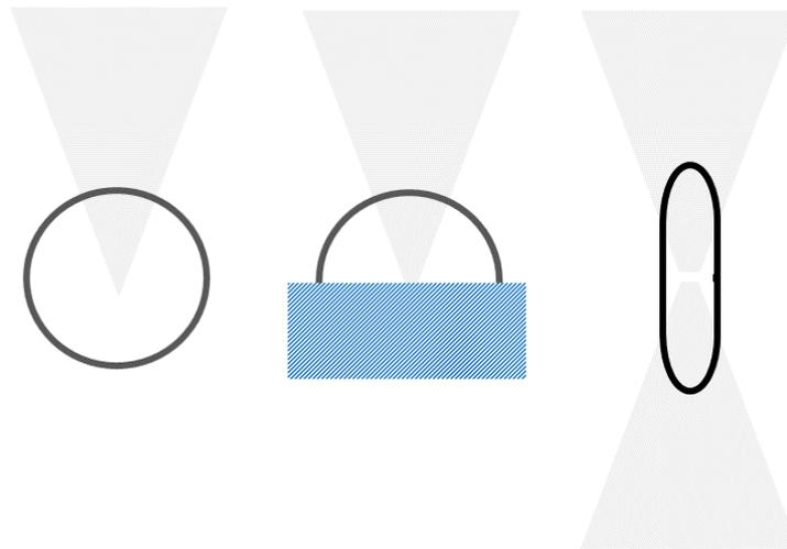
**Figure 1.** Spherical, hemispherical and cylindrical (with hemispherical caps) shock waves induced by a laser in a gas, solid surface or inside a liquid.
