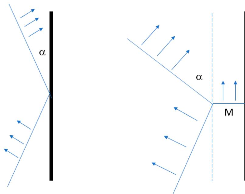
**Figure 4.** Normal reflection of a shock wave (left) vs. Mach wave generation (right). The critical angle  $\alpha$  for the onset of Mach reflection depends on the gas and on the Mach number of the shock wave.
