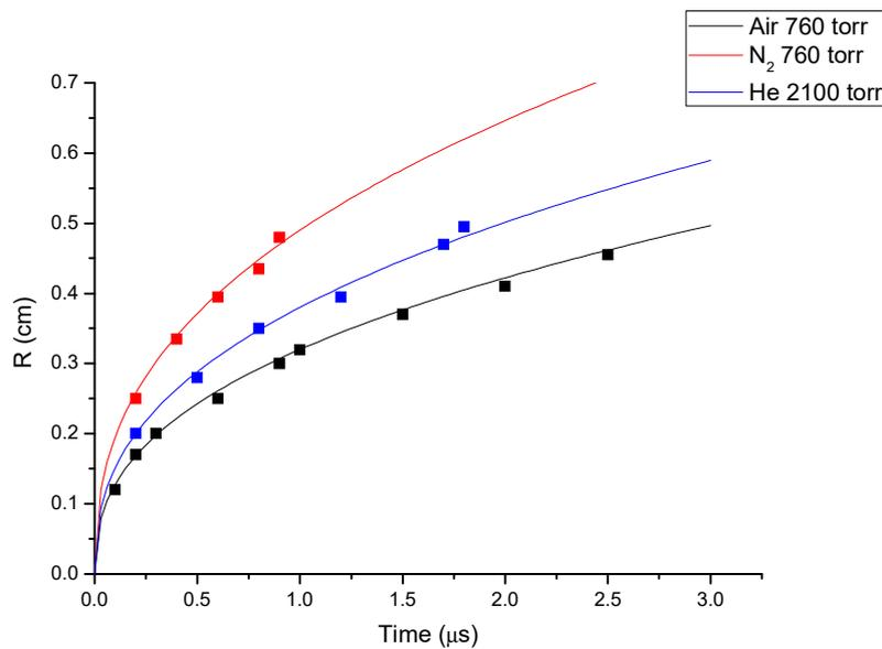
**Figure 3.** Expansion of the spherical shock wave produced by a Nd:YAG laser in gas (black points: Air at pressure of 760 torr; red points: Nitrogen at 760 torr; and blue points: He at 2100 torr). The continuous line represents the predictions of the point strong explosion theory (Equation (1)). The data are from Reference [8].
