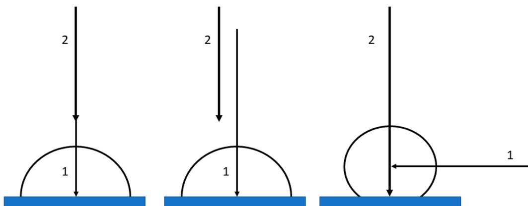
**Figure 6.** Schematic representation of the different double-pulse LIBS schemes where the laser-induced shock wave plays a fundamental role. From the left: Collinear double pulse, parallel double pulse and orthogonal double pulse in pre-ablation configuration.
