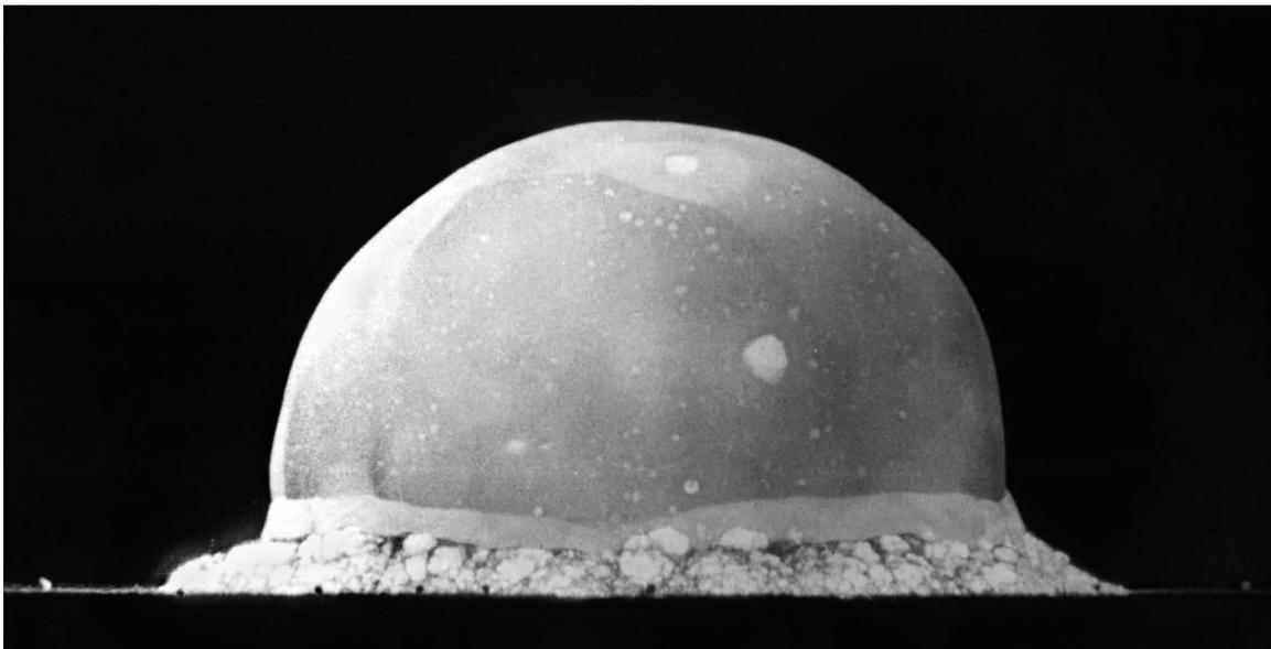
**Figure 2.** The blast wave produced by the first nuclear test, 16 ms after the explosion. The radius of the wave is about 200 m. (Trinity test, New Mexico 1945).
