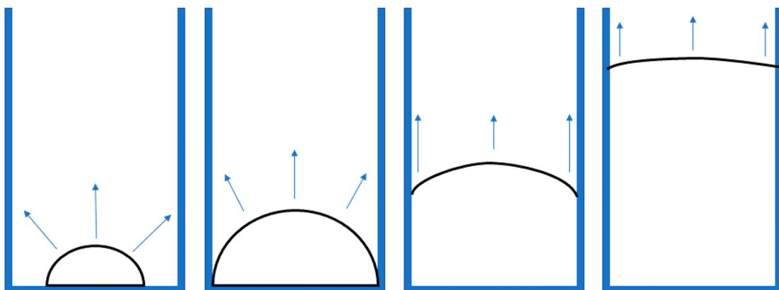
**Figure 5.** Schematic representation of the transformation of a spherical shock wave in a planar one, due to the Mach reflection effect on the walls of a crater. The Mach wave is faster than the initial spherical wave.
