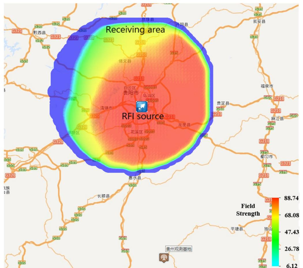
**Figure 5.** The point-to-area analysis for terrestrial RFI source.
