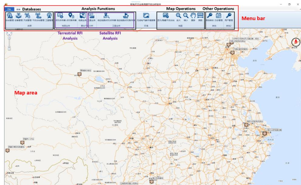
**Figure 3.** The graphical user interface of the RFI analysis software.
