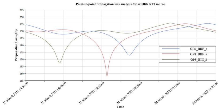
Figure 7. The point-to-point analysis for satellite RFI source.
