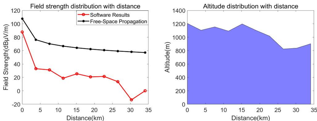
**Figure 4.** The point-to-point analysis for terrestrial RFI source.
