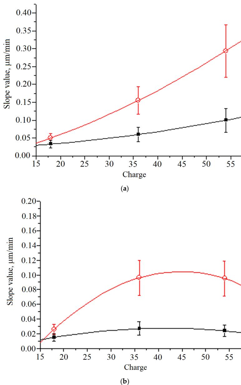
**Figure 4.** Dependence of the slope factors (rates of change in the track dimensions) on the ion charge for large (red line) and small (black line) axis of the ellipses: (a) the etching duration from 30 to 45 min; (b) the etching duration more than 50 min. The experimental points are approximated with parabolas (Color).
