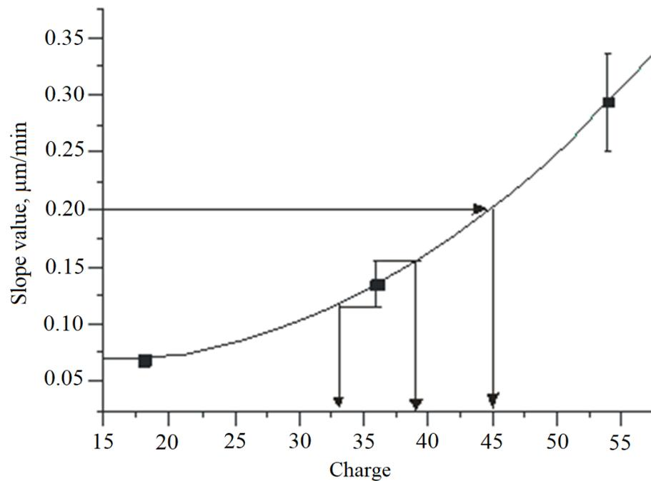
**Figure 5.** Algorithm for the ion charge determining (No color).
