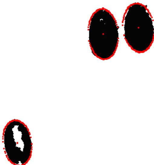
**Figure 2.** Algorithm of the image processing for ion tracks with inclination of  $30^\circ$  to the glass surface. The ion track shape on the surface is parameterized by an ellipse with the PAVICOM software. The image was simulated for ellipse with large axis of 18 microns and small ellipse axis of 11 microns corresponding to xenon tracks (Color).
