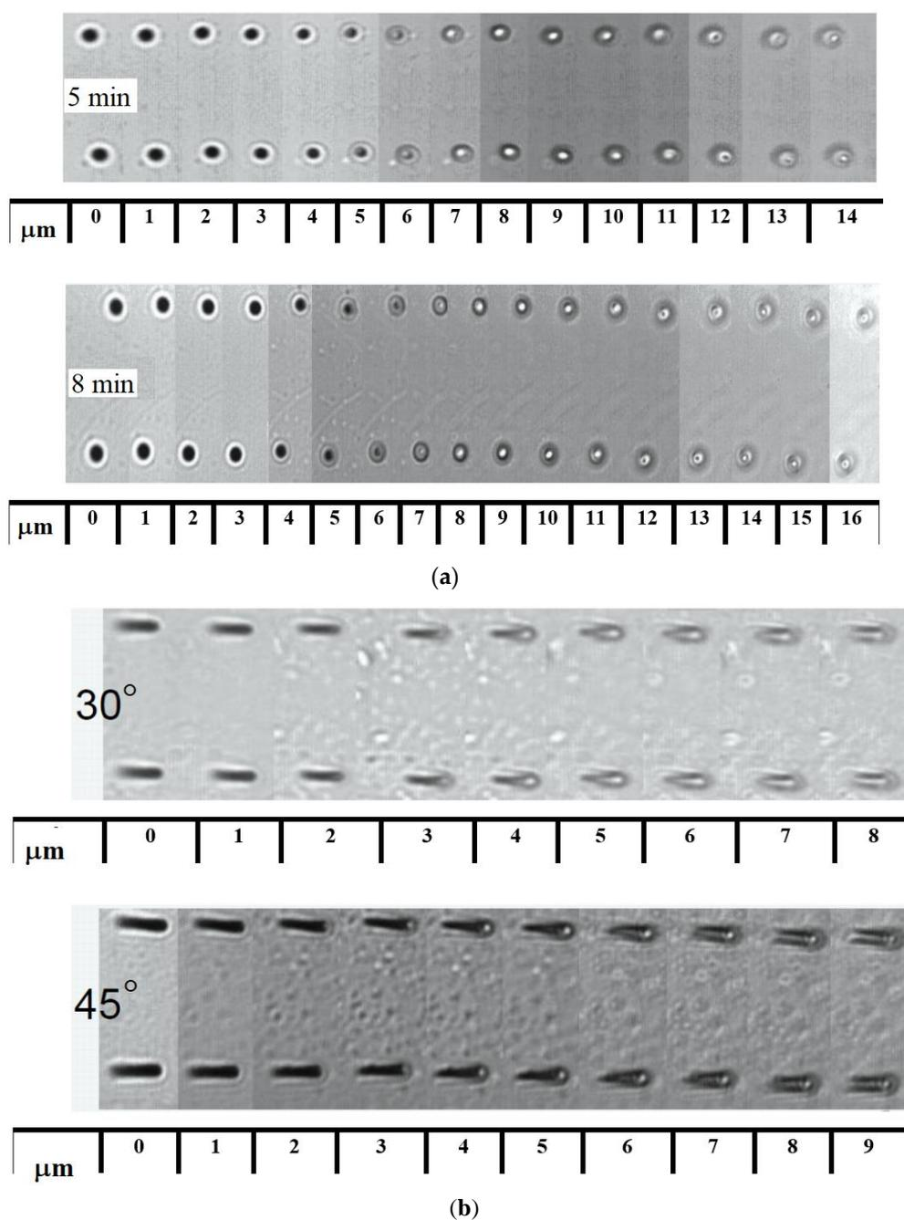
**Figure 1.** The shape of the <sup>132</sup>Xe<sup>26+</sup> ion tracks after etching in 40% HF for different etching depths (indicated under the images): (a) vertical entry, ion energy E = 65–68 MeV (the etching duration is given); (b) entry at 30° and 45° to the normal to the glass surface, ion energy E = 160 MeV; the etching duration is 5 min (No color).
